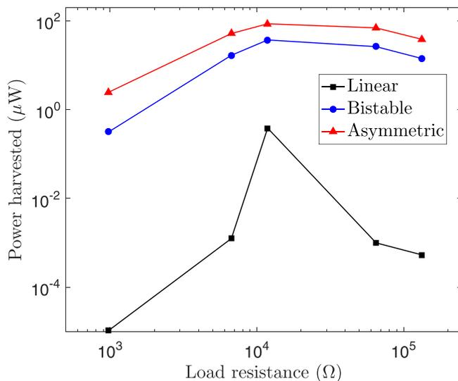
FIG. 6. Variation in the power harvested for different configurations with respect to the load resistance at an excitation level of 0.02 g²/Hz.
