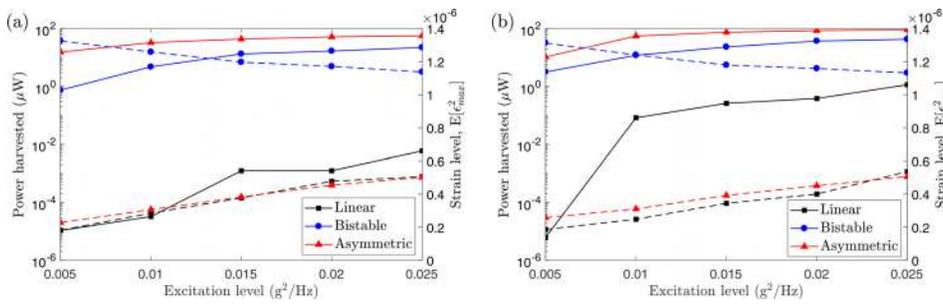
FIG. 5. Variation in the power harvested (represented as solid lines) and the strain level (represented as dashed lines) for different configurations with respect to the excitation amplitude for load resistances of (a) 6.7 kΩ and (b) 11.85 kΩ.
