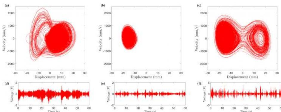
FIG. 4. Experimental phase portraits and voltage time histories corresponding to: (a) and (d) asymmetric harvester at an excitation level of 0.005 g<sup>2</sup>/Hz ( $P = 15.432 \mu\text{W}$ ), (b) and (e) intra-well response of the bistable harvester at 0.005 g<sup>2</sup>/Hz ( $P = 0.749 \mu\text{W}$ ), and (c) and (f) inter-well response of the bistable harvester at 0.02 g<sup>2</sup>/Hz ( $P = 16.812 \mu\text{W}$ ).
