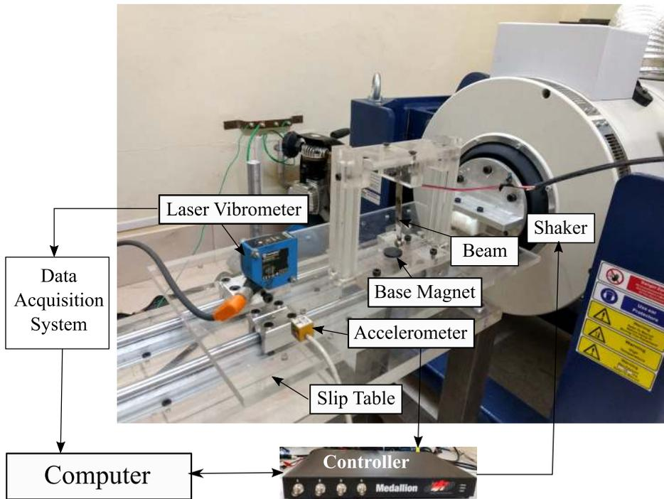
FIG. 3. Experimental test rig, showing the asymmetric energy harvester mounted on a slip table.
