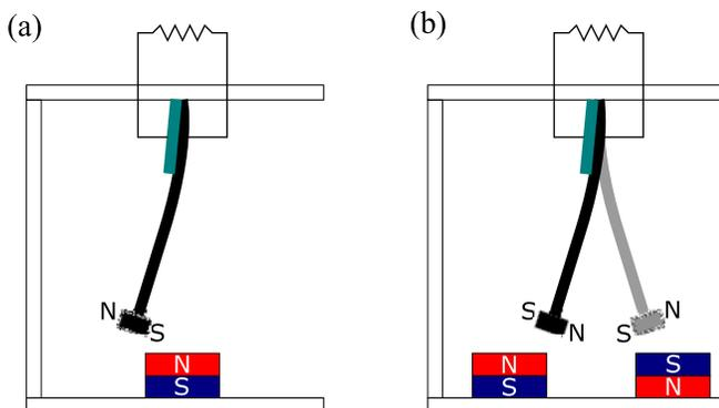
FIG. 1. Schematic representation of the piezomagnetoelastic energy harvester: (a) proposed asymmetric monostable configuration and (b) conventional bistable configuration.
