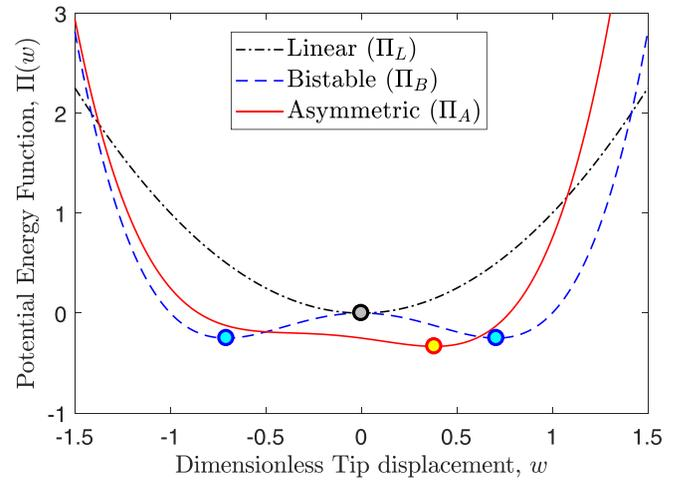
FIG. 2. Potential energy function of the different configurations considered for this study. The static stable equilibrium positions of each configuration are indicated using circle markers of the associated color.
