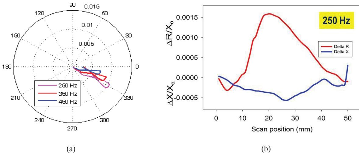
**FIGURE 3.** (a) Coil impedance plane trajectory for a sub-surface notch located 9 mm deep in 10 mm thick aluminium plate. (b) Change in normalized coil impedance at 250 Hz. Defect depth is 1 mm.
