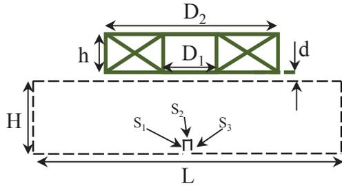
**FIGURE 1.** Coil and sample geometry showing defect surfaces  $S_1$ ,  $S_2$ , and  $S_3$ .
