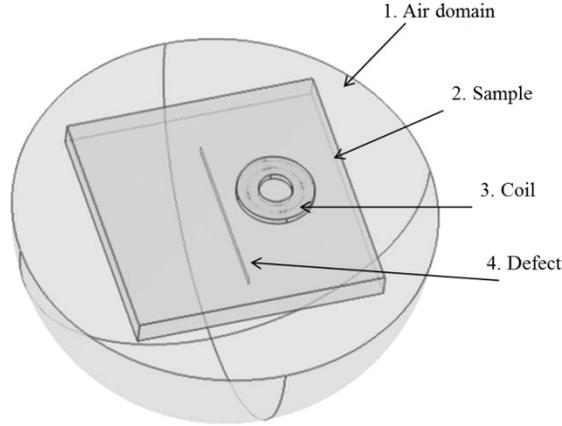
**FIGURE 4.** Schematic of the FEM model
