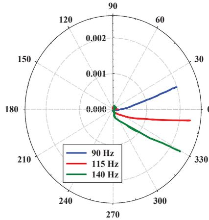
**FIGURE 6.** Impedance plane trajectory of optimized EC coil for 11.5 mm deep 2D notch in 15 mm thick aluminium plate.
