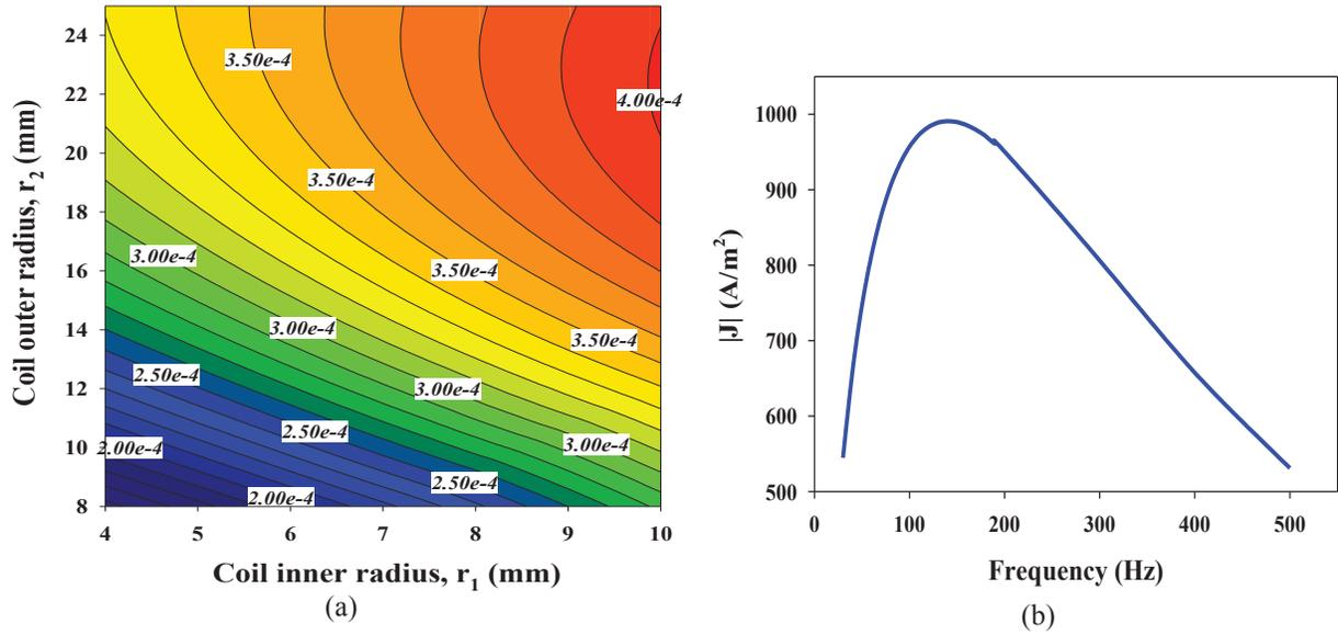
**FIGURE 5.** (a) Magnitude of magnetic field density,  $|\mathbf{B}|$  at 150 Hz on the defect surface ( $S_2$ ) for varying coil inner ( $r_1$ ) and outer ( $r_2$ ) radii, ( $r_1$ : 4 mm to 10 mm;  $r_2$ : 8 mm to 25 mm); (b) induced current density at plate bottom for  $r_1 = 10$  mm,  $r_2 = 23$  mm,  $h = 3$  mm,  $d = 0.5$  mm.
