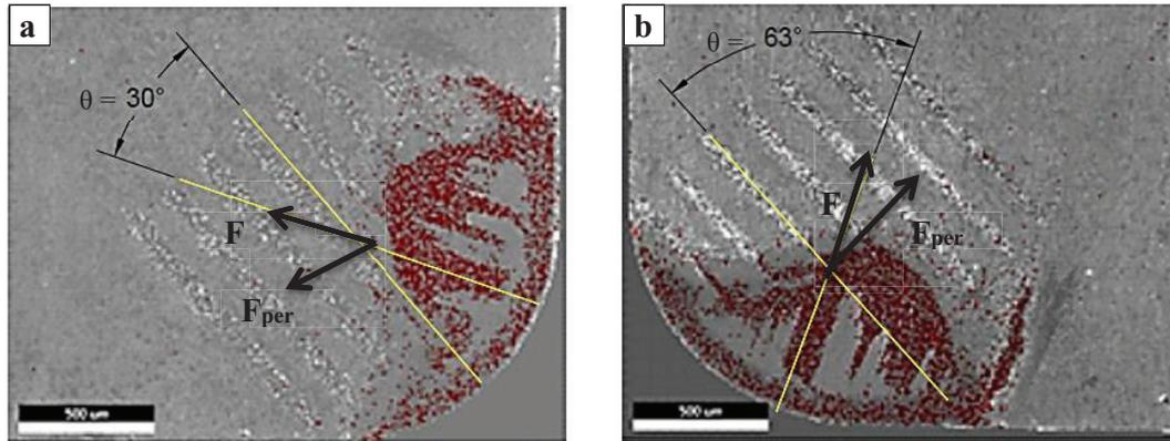
Fig.7. Relative chip flow with respect to lay direction a) PA b) PE tool
