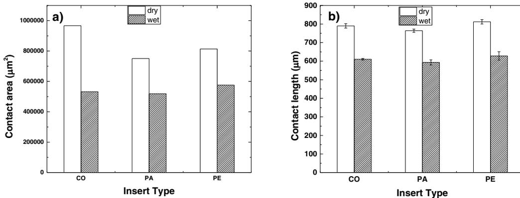
Fig.4. a) Tool chip contact area b) Sticking contact length for all the tools
