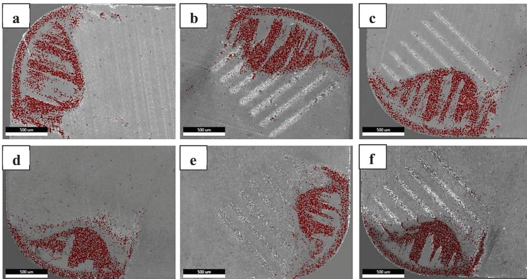
Fig.5. Fe mapping on SEM image of the machined tool inserts a) CO (dry), b) PA (dry), c) PE (dry), d) CO (wet), e) PA (wet) and f) PE (wet)
