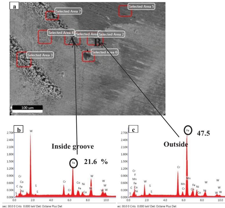
Fig.6. a) SEM image of PA textured tool (wet) and corresponding EDS analysis for (b) area A inside groove and (c) area B outside groove
