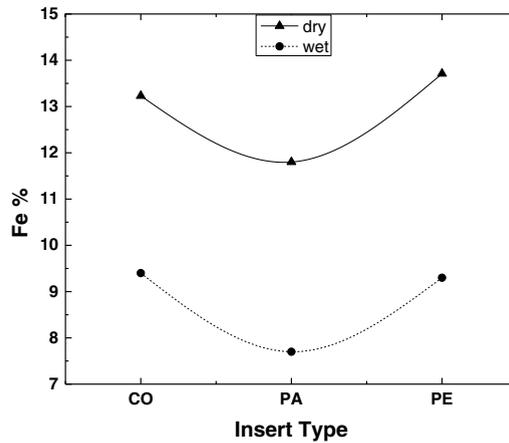
Fig.3. Fe deposition % for different cutting tool inserts
