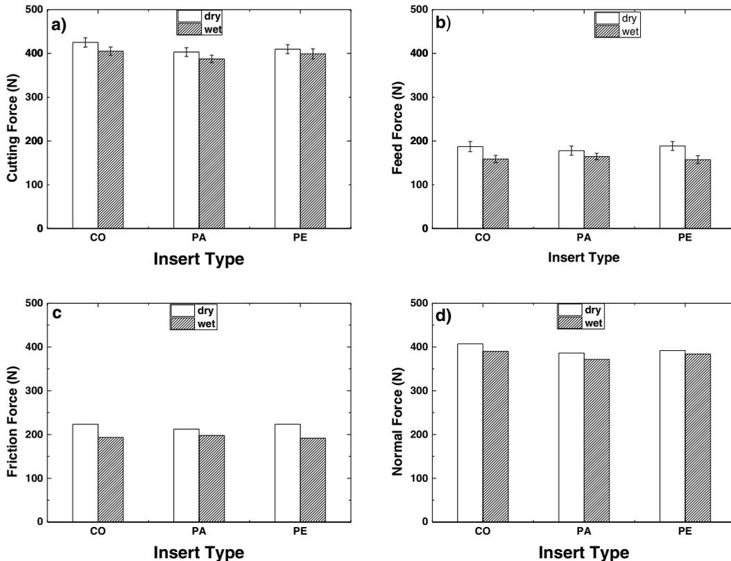
Fig.2. a) Cutting force b) feed force c) friction force d) normal force for different tools
