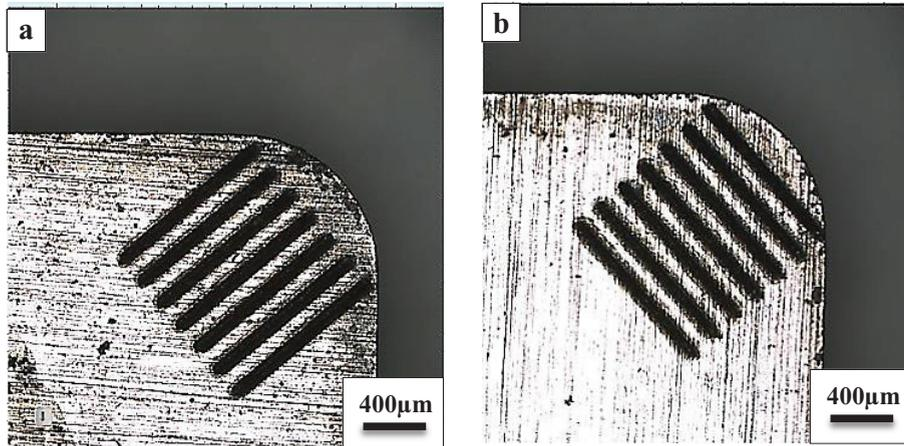
Fig.1. Optical images of micro scale textured tool a) parallel to chip flow (PA) and b) perpendicular to chip flow (PE)
