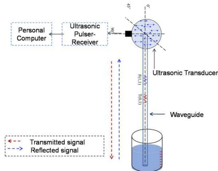
Figure 7. Experimental setup schematic for level measurement experiments.
