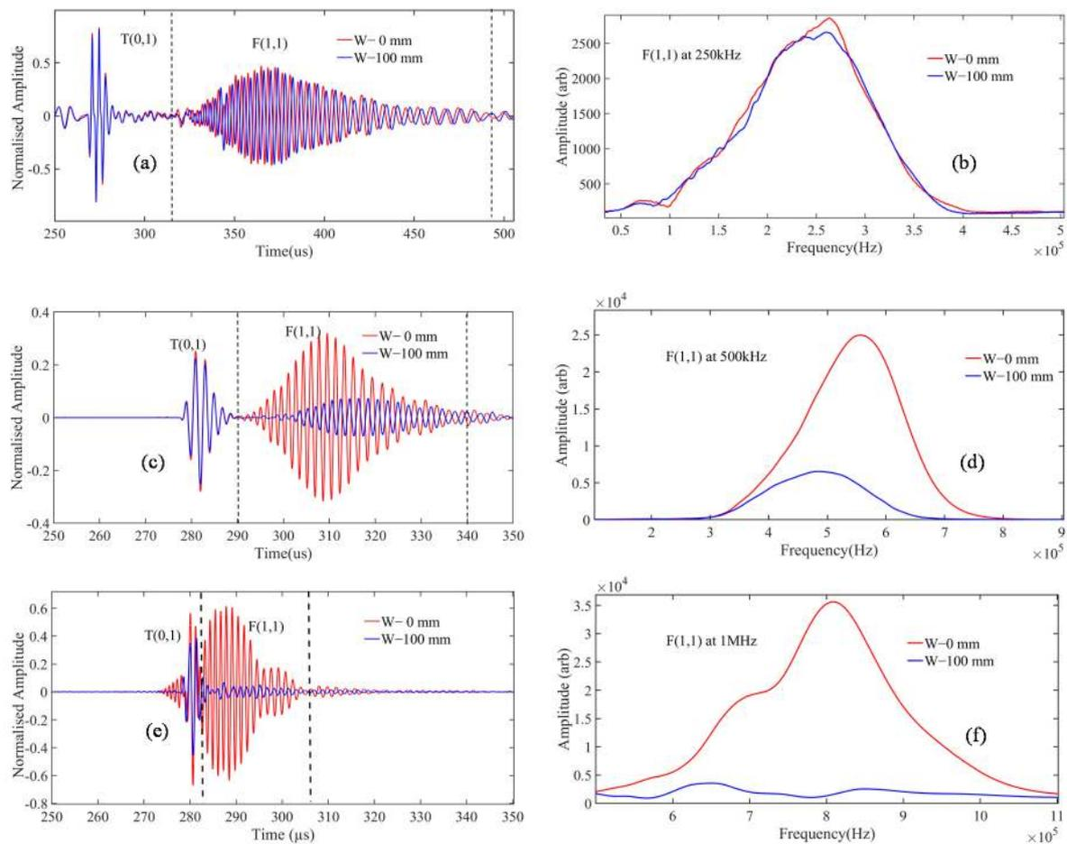
**Figure 8.** Obtained A-Scan signal at 0 cm and 10 cm fluid loading at the frequencies of (a) 250 kHz, (c) 500 kHz, and (e) 1000 kHz and their corresponding FFT plots at (b) 250 kHz, (d) 500 kHz, and (f) 1000 kHz.
