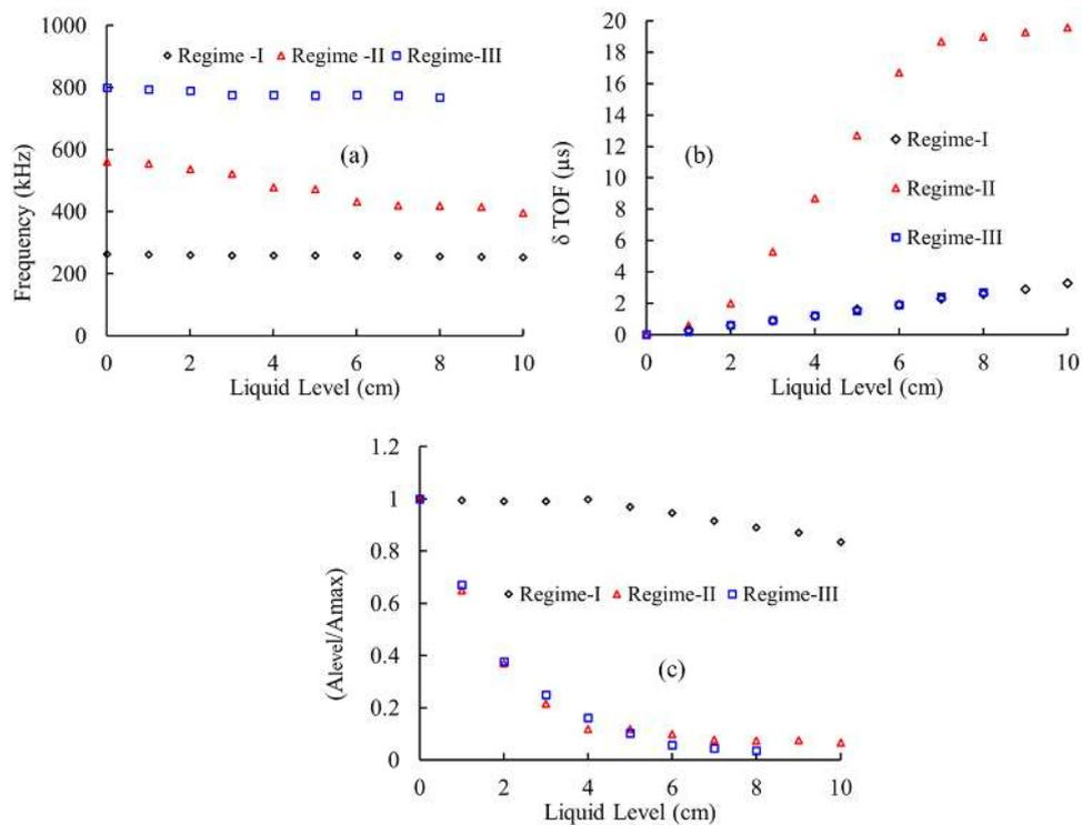
**Figure 9.** Illustrates the (a) shift in peak frequency, (b) change in time of flight ( $\delta$ TOF), and (c) drop in amplitude of F(1,1) wave modes at different fluid levels in Regime-I (250 kHz), Regime-II (500 kHz), and Regime-III (1000 kHz).
