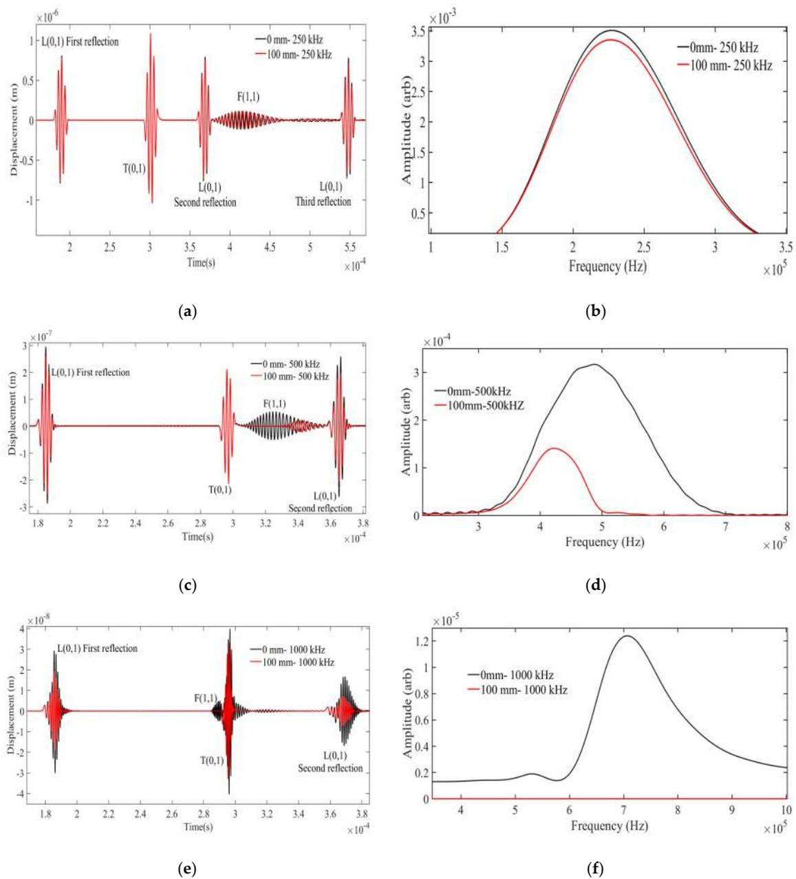
**Figure 6.** A-Scan signals at the frequencies of (a) 250 kHz, (c) 500 kHz, and (e) 1000 kHz at a  $45^\circ$  angle of excitation and their corresponding FFT plots of F(1,1) at (b) 250 kHz, (d) 500 kHz, and (f) 1000 kHz.
