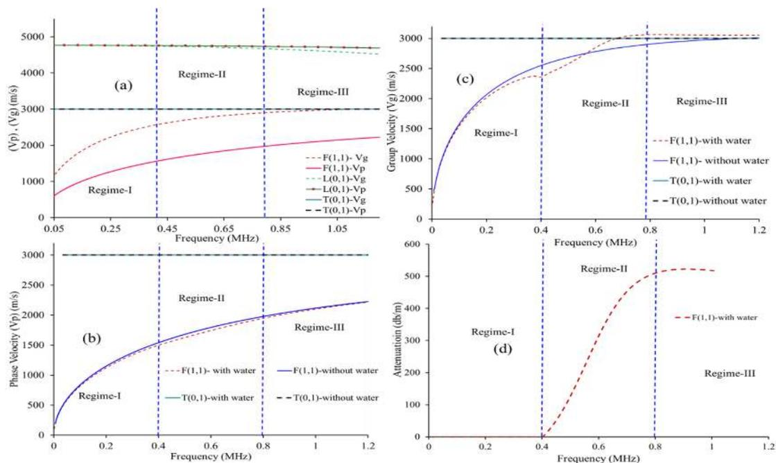
**Figure 1.** (a) Dispersion curves of 1.00 mm dia SS-308L waveguide in free boundary conditions (phase velocity ( $V_p$ ) and group velocity ( $V_g$ )), [(b,c)]  $V_p$  and  $V_g$  at fluid (water) loaded, (d) Attenuation plot in water loaded condition.
