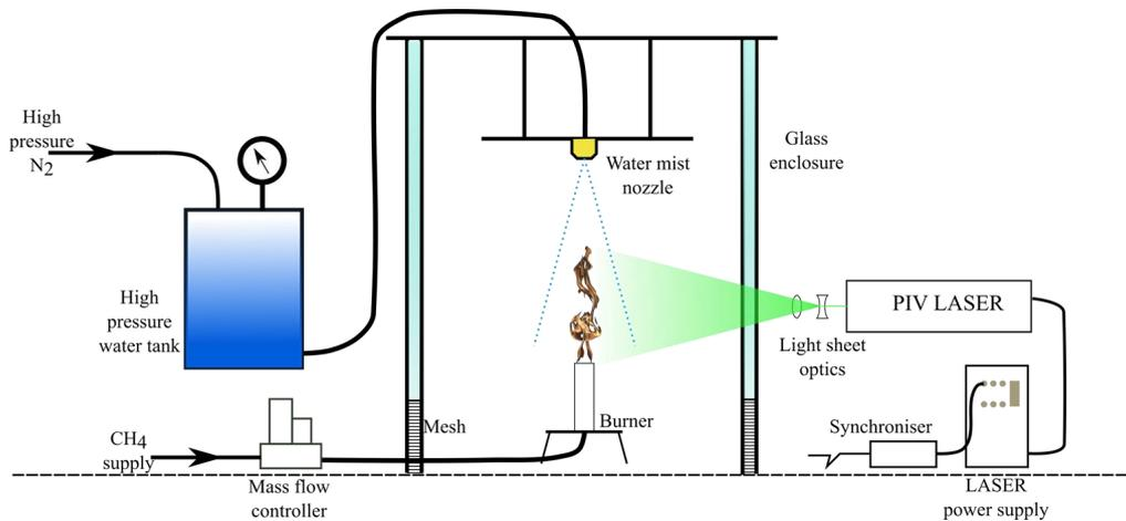
Fig.1. Schematic of the experiment; the sketch is not to scale.
