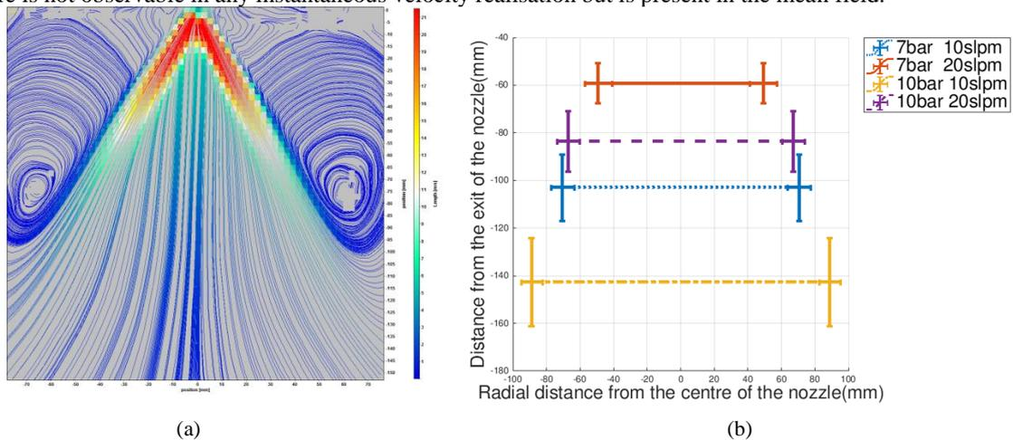
Fig.4. Representation of the re-circulation zone for 7bar spray suppressing a 20slpm flame and the location-size statistics of the vortex.
