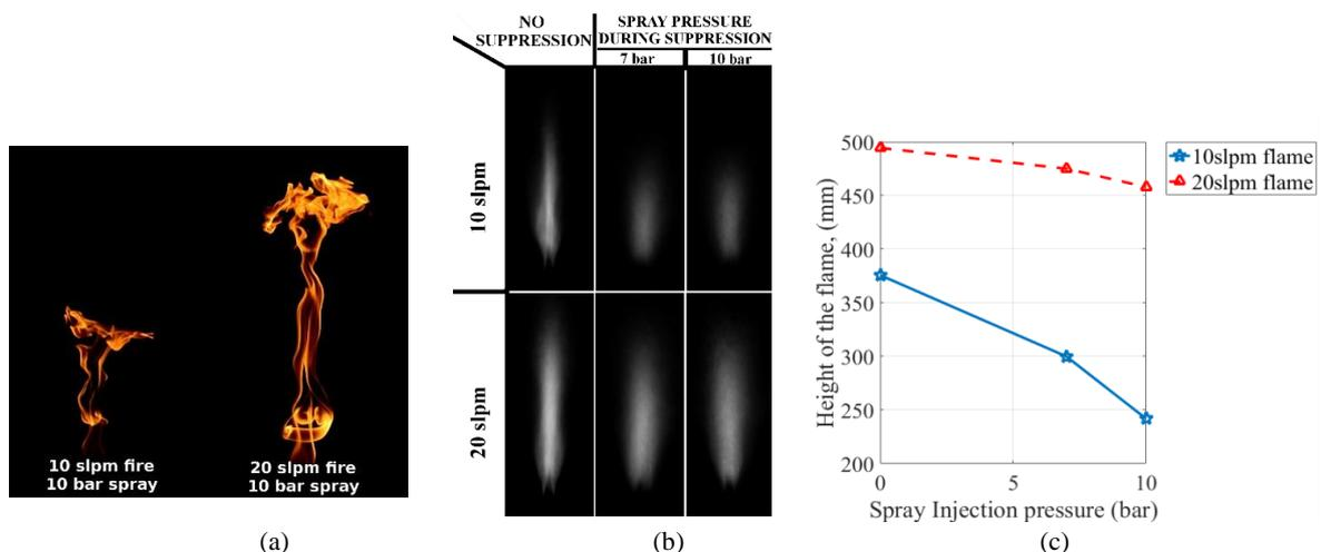
Fig. 2a Instantaneous Flame tip flattening, Fig.2b Changes to the flame luminosity, Fig.2c Flame height trend
