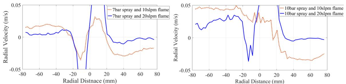
Fig.5.Radial profile of the Radial velocity component, 80mm above the burner.
