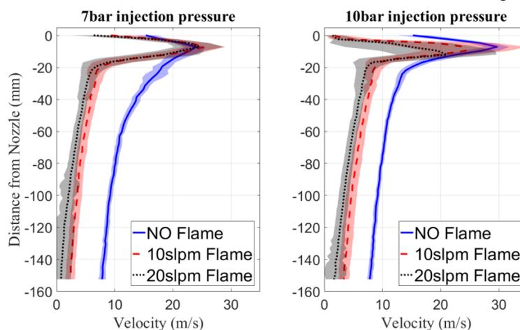
Fig. 3. Centreline velocity magnitude profile of the spray, with and without flame.
