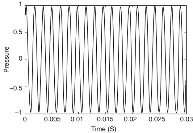
**Figure 10:** Time trace of acoustic pressure signal corresponding to second mode limit cycle oscillations (region IV of Fig. 3) for an input heat flux of 190 Watts. Note that all the local maxima have same amplitude. Also, the pressure values are normalized.
