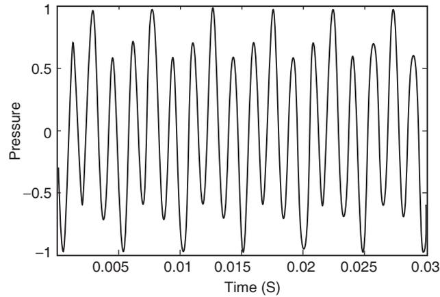
**Figure 7:** Time trace of acoustic pressure signal corresponding to quasiperiodic oscillations (region III of Fig. 3) for an input heat flux of 160 Watts. Note that the local maxima have different amplitude. Also, the pressure values are normalized.
