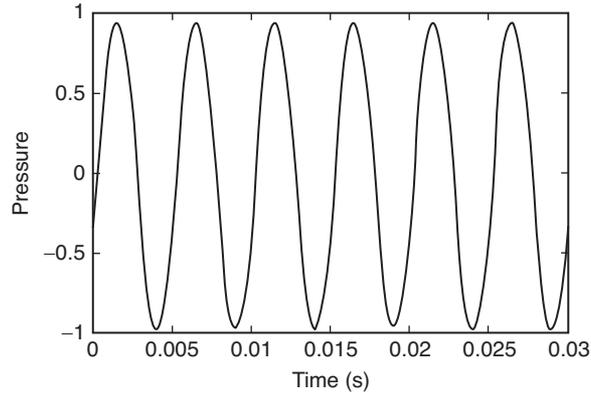
**Figure 4:** Time trace of acoustic pressure signal corresponding to limit cycle oscillations (region II of Fig. 3, fundamental mode) for an input heat flux of 72 Watts. Note that all the local maxima have same amplitude. Also, the pressure value is normalized.
