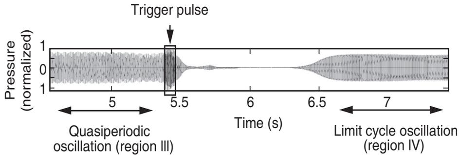
**Figure 13:** Transition of quasiperiodic oscillation to limit cycle oscillation through triggering. An acoustic signal (trigger pulse) was used to enable triggering. The trigger pulse was produced using an acoustic driver. The pulse had a frequency of 200 Hz, a width of 0.1s and an amplitude roughly 1.3 times the amplitude of self-excited oscillation.
