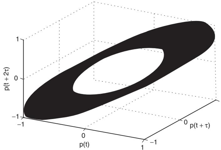
**Figure 9:** Phase portrait corresponding to quasiperiodic oscillations (region III of Fig. 3). Here, the input heat flux is 160 Watts and the pressure values are normalized.
