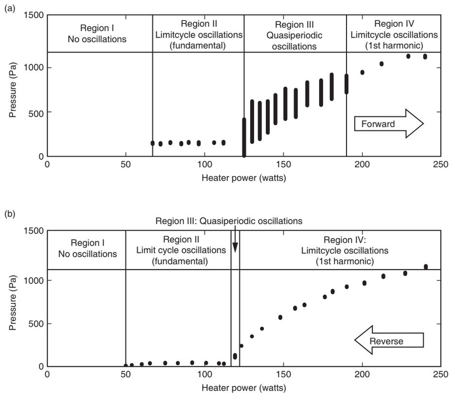
**Figure 3:** Bifurcation diagram. Local maxima of each cycle in the pressure signal are plotted for each heater power location. a) Increasing heat flux (Forward direction). b) Decreasing heat flux (Reverse direction). Comparing the forward and reverse path of the bifurcation diagram, it is evident that there is hysteresis in the bifurcation. This is indicative of a subcritical bifurcation.
