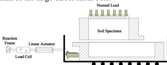
Fig.1. A schematic of large shear box showing major components.
