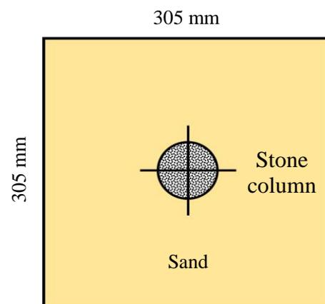
Fig. 3. Schematic diagram of single stone column at the center of shear box.
