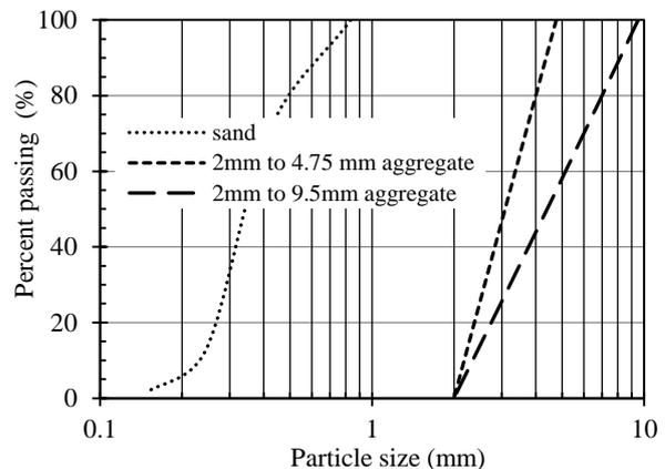
Fig.2. Grain size distribution of sand and aggregates.
