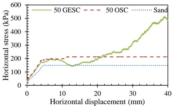
Fig. 7. Horizontal stress ( $\sigma_x$ ) developed above the shear plane.
