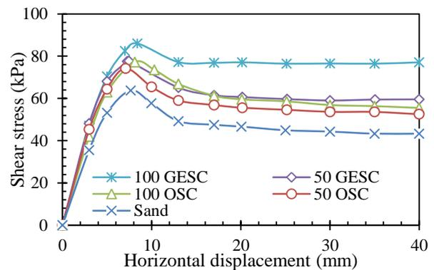
Fig. 5. Shear stress vs. displacement ( $\sigma_n = 75$  kPa).
