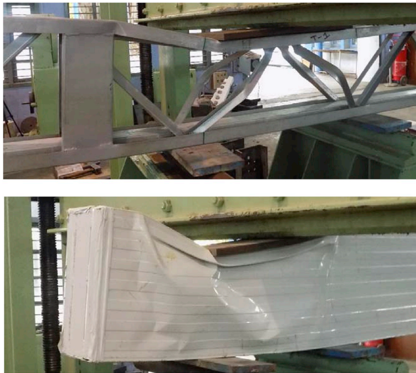
Fig. 11. Observed failure of specimens S-B1-BF and S-B2-F/PUF (shear).
