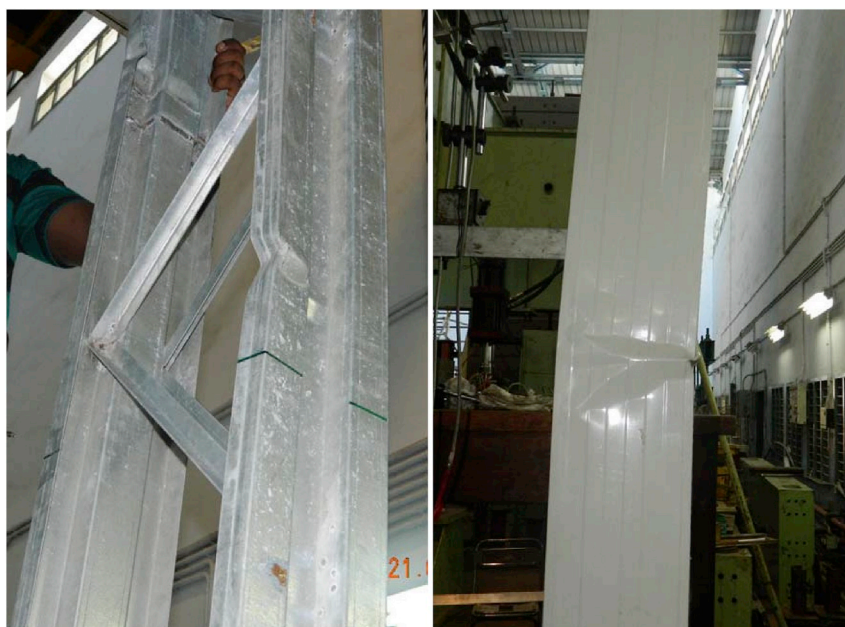
Fig. 12. Observed failure of specimens C-B1-BF and C-B2-F/PUF (axial compression).
