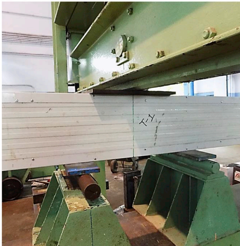
Fig. 4. a)Schematic experimental test set-up: shear, b)Photograph of experimental test set-up: shear.
