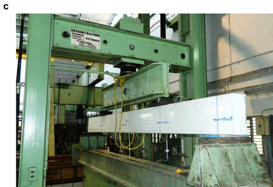
Fig. 3. a) Schematic experimental test set-up: flexure, b) Photograph of experimental test set-up: flexure (specimen: F-B1-BF-XX), c) Photograph of experimental test set-up: flexure (specimen: F-B2-F/PUF-XX).
