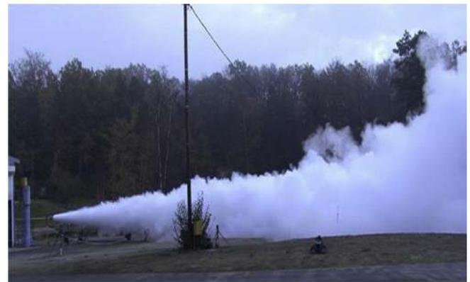
Fig. 2. INERIS Test 8 showing the vapour cloud. The vertical column shown is at a distance of 10 m downstream from the orifice.
