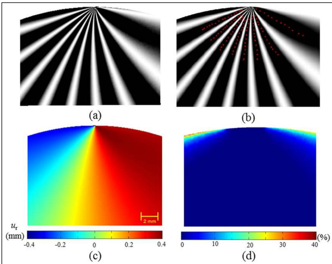
**Figure 4.** Pseudo fringes of radial displacement from (a) experimental results from DIC, (b) reconstructed using the parameters obtained from the nonlinear least squares method with data points echoed back, (c) contour plot of the  $u_r$  displacement shown in (b) and (d) error plot of  $u_r$  displacement.
