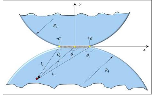
Figure 1. Schematic diagram of the contact zone of two discs in contact.
