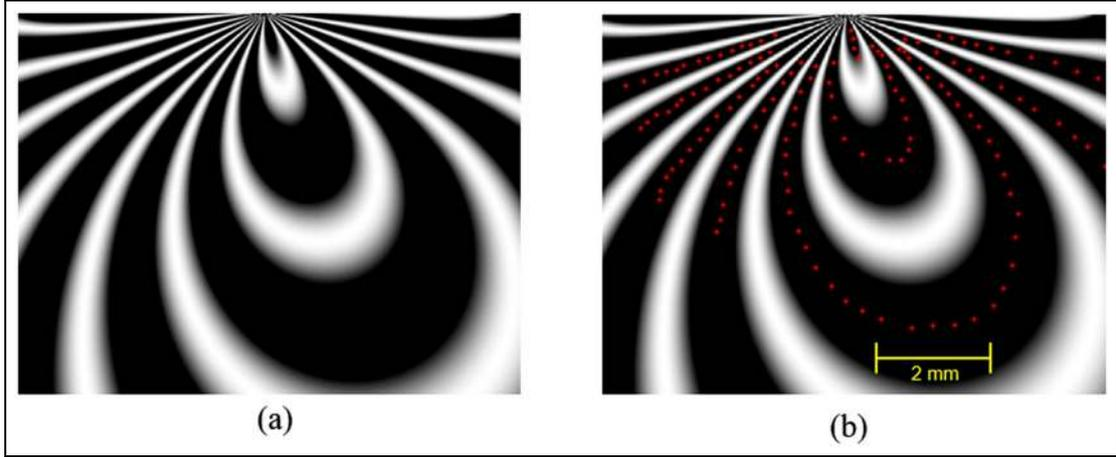
**Figure 2.** Pseudo fringes of radial displacement ( $M=40$ ) from (a) analytical data for  $a=3$ ,  $T_x=0.1$ ,  $T_y=-0.5$  and (b) reconstructed using the parameters obtained from the nonlinear least squares method with data points echoed back.
