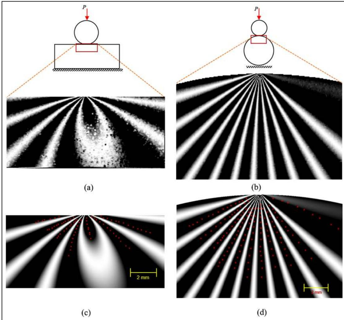
**Figure 5.** Pseudo fringes of radial displacement from experimental DIC results for (a)  $\eta = 1.85/R$ , (b)  $\eta = 2.85/R$ . Reconstructed using the parameters obtained from the nonlinear least squares method with data points echoed back for contact zone with (c)  $\eta = 1.85/R$  and (d)  $\eta = 2.85/R$ .
