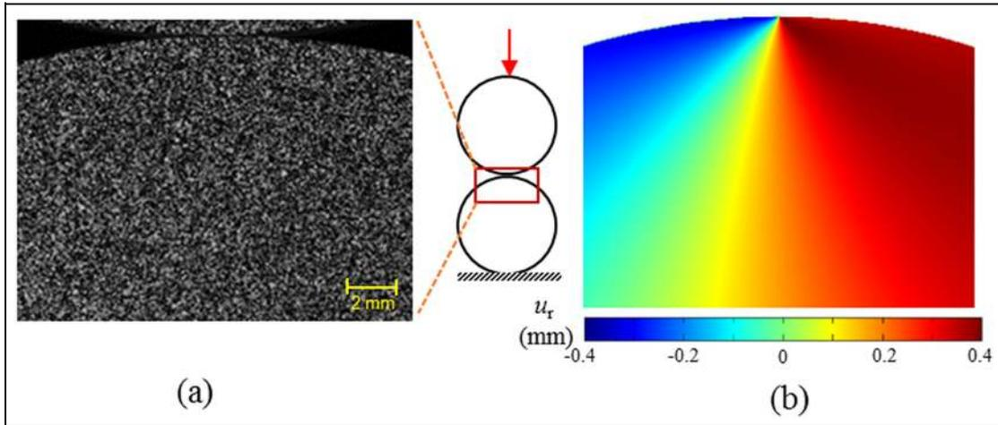
**Figure 3.** (a) Speckled model for reference image and (b) contour plot of the  $u_r$  displacement obtained from DIC analysis.
