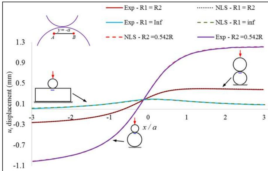
**Figure 6.** Variation of the radial displacement along  $x/a$  at  $y=-a$  for experimental and least squares model for three cases of contacting situations.
