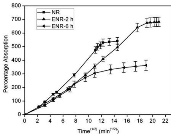
**Fig. 7** Percentage absorption (% w/w) of petrol vs. time<sup>(1/2)</sup> for NR, ENR-2 h and ENR-6 h.
