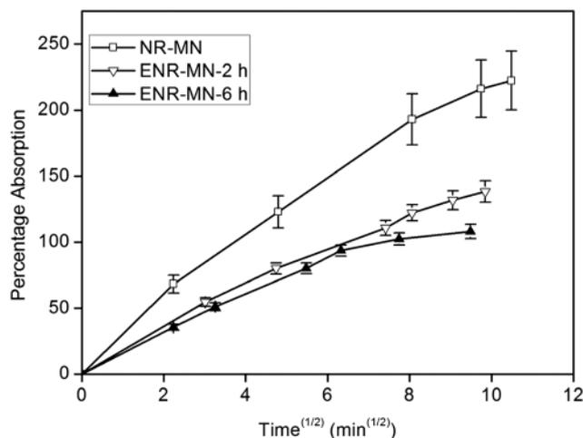
**Fig. 8** Percentage absorption (% w/w) of petrol vs. time<sup>(1/2)</sup> for NR-MN, ENR-MN-2 h and ENR-MN-6 h.
