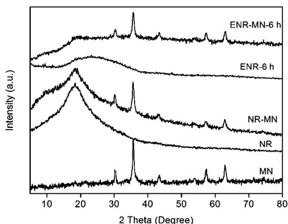
Fig. 5 X-ray diffraction spectra of the MN, NR, ENR-6 h and the nanocomposites.
