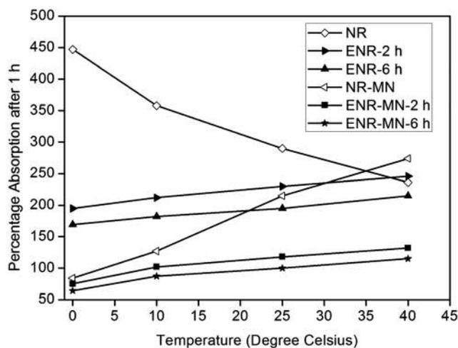
Fig. 11 Effect of temperature versus % petrol absorption plots for all the absorbents.
