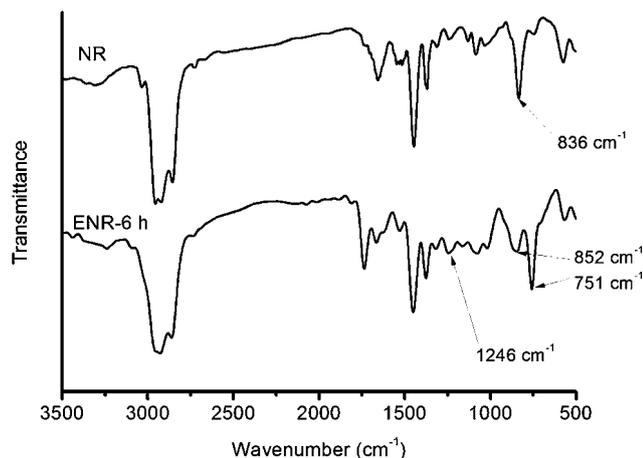
Fig. 2 FTIR spectra of NR (above) and ENR-6 h (below).
