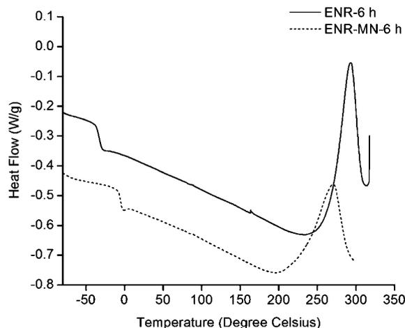
Fig. 4 DSC curves of ENR-6 h and ENR–MN-6 h (heating rate  $10\text{ }^{\circ}\text{C min}^{-1}$ ).
