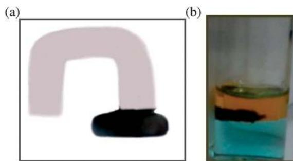
**Fig. 9** (a) ENR-MN, post-petrol absorption attracted by a magnet; (b) ENR-MN, post-petrol absorption floating at the petrol-water interface as contrasted by the addition of CuSO<sub>4</sub> to the aqueous layer.
