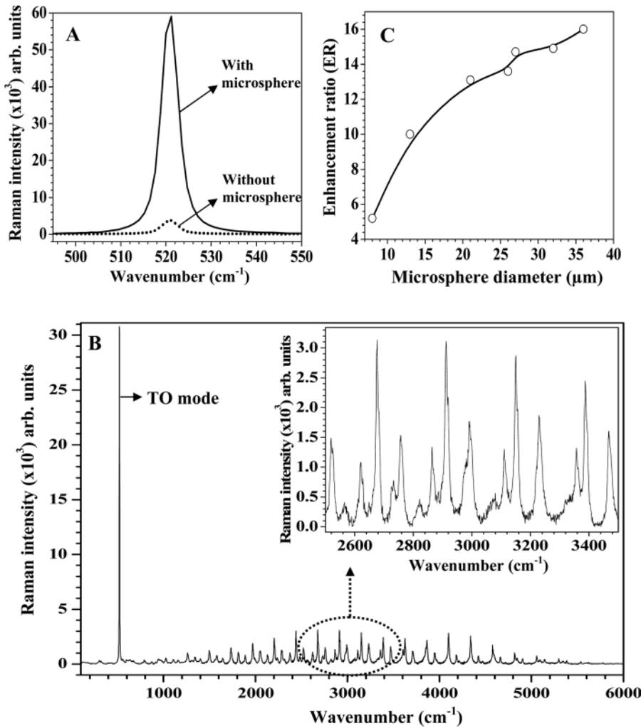
FIG. 3. (A) Enhancement of Raman intensity of the  $521\text{ cm}^{-1}$  peak of silicon wafer (with microsphere of diameter  $\sim 36\ \mu\text{m}$ ). Typical Raman spectrum of silicon wafer on exciting through a single silica microsphere of diameter  $\sim 10\ \mu\text{m}$  (B). The inset shows an expanded region of the spectrum showing WGMs. Panel C shows the ER obtained with single silica microspheres.
