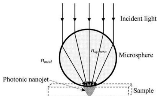
FIG. 2. Schematic of the photonic nanojet emerging from a single microsphere.
