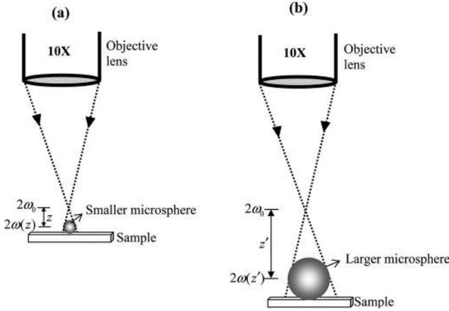
FIG. 1. The schematic of the experimental setup for enhancement of Raman scattering signal of the sample with (a) smaller and (b) larger microsphere. Here,  $2\omega_0$  is the beam diameter at the focal point.  $2\omega(z)$  and  $2\omega(z')$  are the beam diameters at the distances  $z$  and  $z'$ , respectively.
