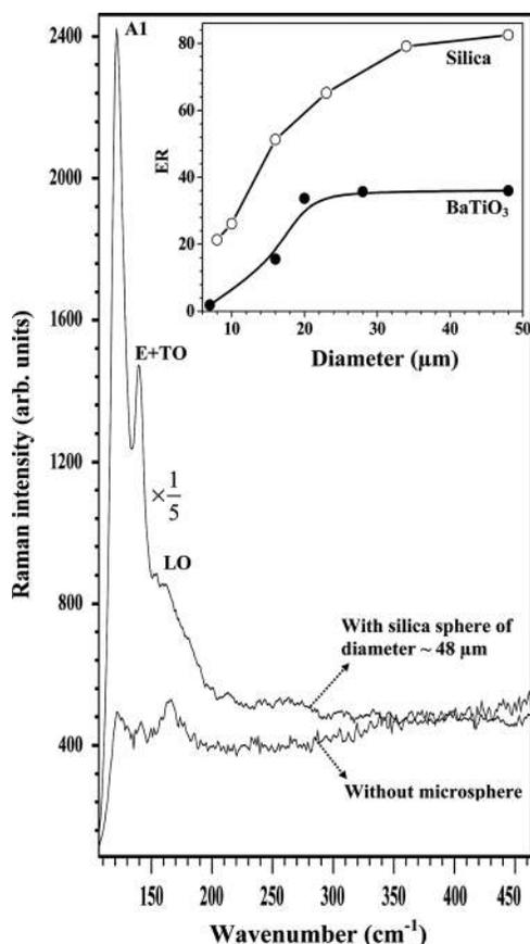
FIG. 4. Raman spectra of CdTe<sub>2</sub> thin film obtained with the excitation wavelength of 632.8 nm through the 10 × lens. Inset shows the obtained ER of the A1 peak with the different microspheres.
