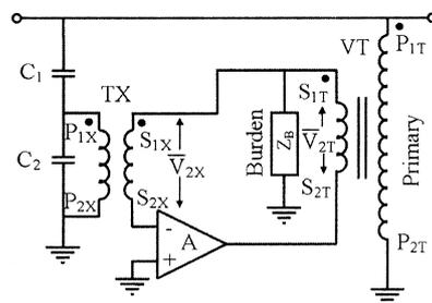
Fig. 1. Electronic error compensation for a VT using high gain amplifier
