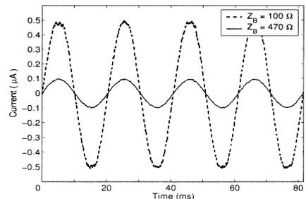
Fig. 4. Measured current through the voltage follower for scheme of Fig. 2
