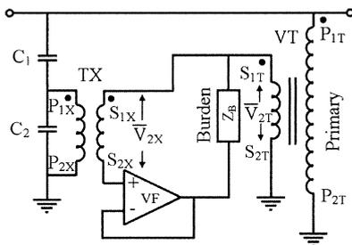
Fig. 2. Electronic error compensation for a VT using unity gain amplifier
