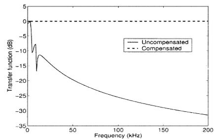
Fig. 3. Frequency response of voltage transformer by simulation
