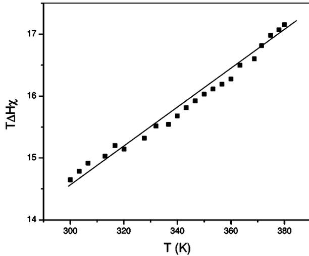
FIG. 4. Temperature dependence of the product  $T\Delta H\chi$  for NSMO (0.3) crystal. Solid line is a guide to the eye.
