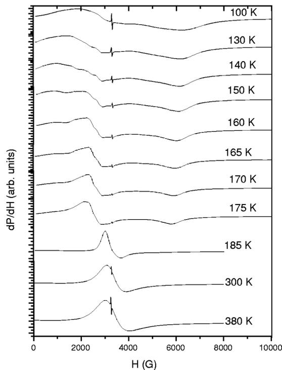
FIG. 1. ESR spectra of NSMO (0.3) crystal in the paramagnetic state and ferromagnetic state.
