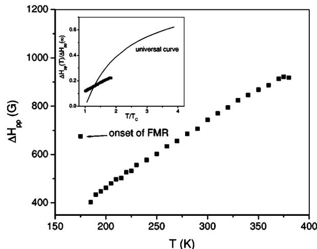
FIG. 3.  $\Delta H_{\text{pp}}$  vs temperature for NSMO (0.3) single crystal. Inset shows  $\Delta H_{\text{pp}}(T)/\Delta H_{\text{pp}}(\infty)$  vs temperature for NSMO (0.3) and universal dependence of  $\Delta H_{\text{pp}}(T)/\Delta H_{\text{pp}}(\infty)$  for manganites.
