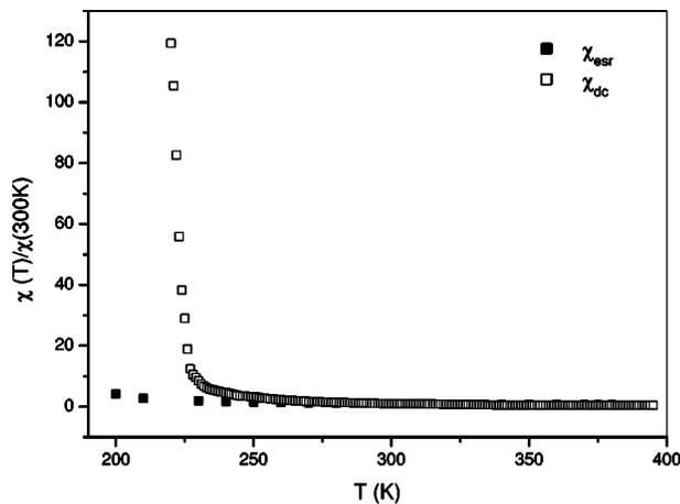
FIG. 5. Temperature dependence of  $\chi_{\text{esr}}$  and  $\chi_{\text{dc}}$  of NSMO (0.3) crystal normalized to  $\chi(300\text{ K})$ .
