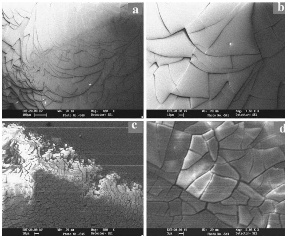
FIG. 4. (a) SEM image of the as-deposited tungsten oxide thin film showing layered structure along the edge of the film. (b) Extended view of the layered structure in S1. (c) The low magnification image of the electron bombarded sample S3. (d) High-magnification SEM image of sample S3 showing cracks at the point of electron impingement.
