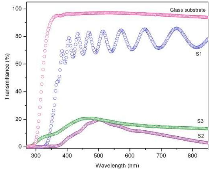
FIG. 2. (Color online) The spectral dependence of transmittance in the wavelength range 250–850 nm for the as-deposited (S1) and electron bombarded (S2, S3) WO<sub>3</sub> thin films.
