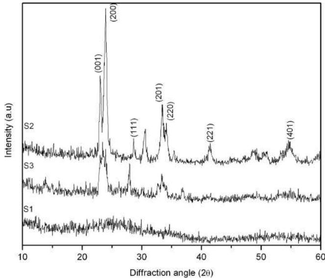
FIG. 1. X-ray diffraction pattern of the as deposited (S1) and electron bombarded (S2, S3) tungsten oxide thin films deposited by pulsed dc magnetron sputtering.
