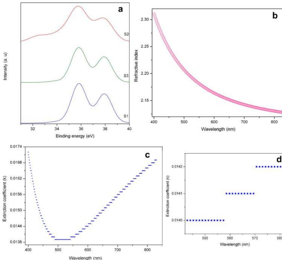
FIG. 3. (Color online) (a) XPS spectrum of the as-deposited (S1) and electron bombarded (S2, S3) WO<sub>3</sub> thin films in the region of W 4f levels. (b) Refractive index of sample S1 as a function of wavelength. (c) Spectral dependence of extinction coefficient for the as-deposited tungsten oxide thin films. (d) Extended view of *k* values showing the individual data points in each step.
