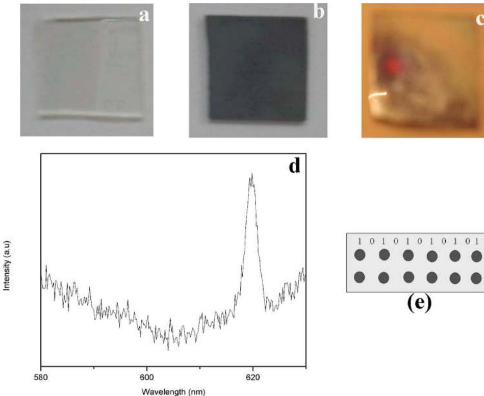
FIG. 6. (Color online) The photographs of the (a) as-deposited sample S1; (b) colored sample S2; and (c) light-emitting sample S3. (d) The PL spectrum of sample S3 excited at  $\lambda = 325$  nm. (e) Outline for data storage application based on the coloration/luminescence of  $WO_3$  thin films by electron bombardment.
