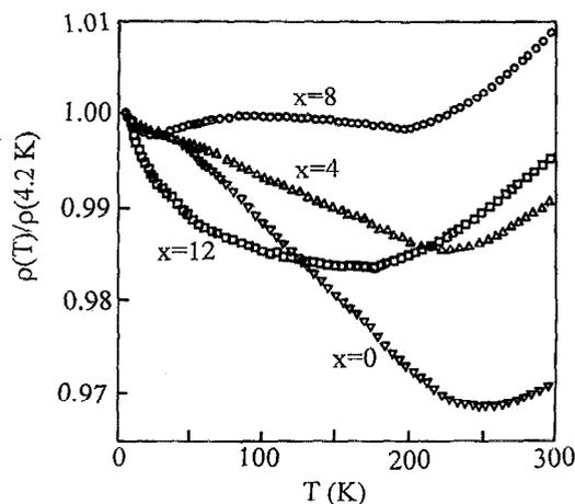
FIG. 1.  $\rho(T)/[\rho(4.2\text{ K})]$  as a function of temperature for  $\alpha$ - $\text{Fe}_{90-x}\text{Mn}_x\text{Zr}_{10}$  with  $x=0, 4, 8,$  and  $12$ .
