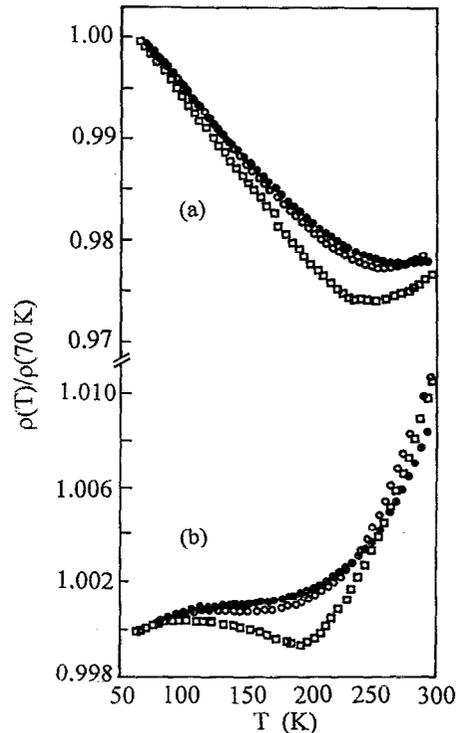
FIG. 3. Normalized resistivity,  $\rho(T)/\rho(70\text{ K})$ , as a function of temperature for  $a\text{-Fe}_{90-x}\text{Mn}_x\text{Zr}_{10}$  with (a)  $x=0$  and (b)  $x=8$  for different values of the applied magnetic field: 0 T (■); 0.7 T (○); and 4.0 T (●).
