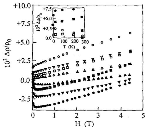
FIG. 4.  $\Delta\rho/\rho_0 = [\rho(H, T) - \rho(0, T)] / [\rho(0, T)]$  as a function of applied magnetic field for  $x=0$  (●, ○);  $x=4$  (▼, ▽);  $x=8$  (■, □); and  $x=12$  (▲, △). Closed symbols represent the transverse mode and open symbols represent the longitudinal mode. Inset: magnetoresistance as a function of temperature for  $x=0$  (closed symbols) and  $x=8$  (open symbols) in an applied field of 0.7 T (□, ■) and 4.0 T (○, ●).
