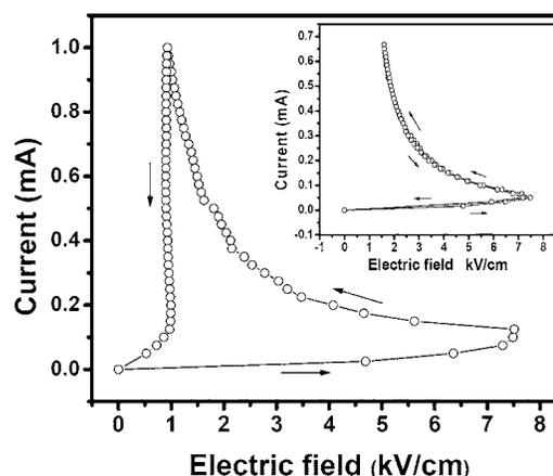
FIG. 1. *I-V* characteristics of Ge<sub>15</sub>Te<sub>83</sub>Si<sub>2</sub> glass with 1 mA input current showing memory switching. The inset shows the *I-V* characteristics of the sample with 0.7 mA input current (threshold behavior).
