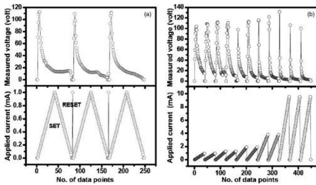
FIG. 2. (a) *set/reset* operations in  $\text{Ge}_{15}\text{Te}_{83}\text{Si}_2$  glass carried out using a triangular (*set*) and a rectangular (*reset*) pulse of 1 mA amplitude. (b) Electrical switching behavior of  $\text{Ge}_{15}\text{Te}_{83}\text{Si}_2$  glass obtained with a saw-tooth current pulse.
