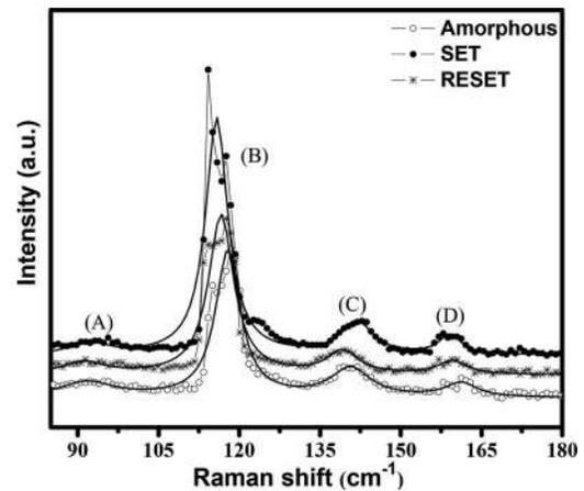
FIG. 3. *In situ* Raman spectrum of  $\text{Ge}_{15}\text{Te}_{83}\text{Si}_2$  sample in (a) amorphous, (b) *set*, and (c) *reset* states.
