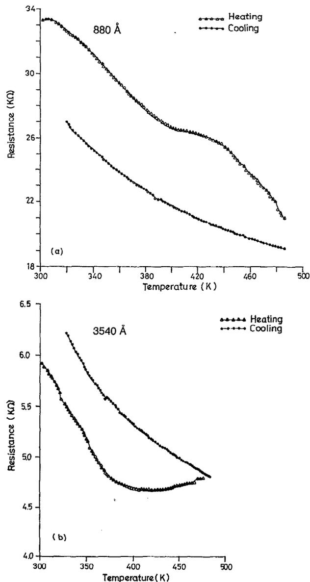
FIG. 1. Resistance variation during heating-cooling cycles of typical as-grown thin films of  $\text{Ga}_5\text{Se}_{20}\text{Te}_{75}$  (thickness 880 Å and 3540 Å).
