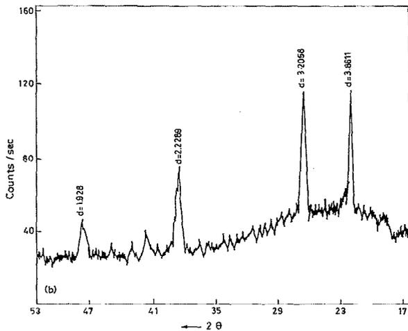
FIG. 2. (a), (b) X-ray patterns of the typical as-grown thin film before and after resistance measurements.
