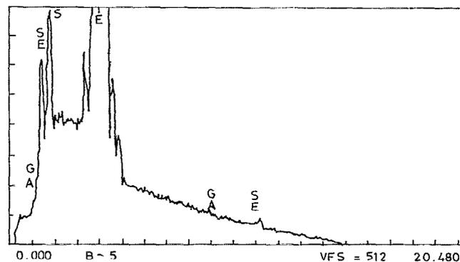
FIG. 5. EDAX pattern of a typical thin film of  $Ga_5Se_{20}Te_{75}$ .
