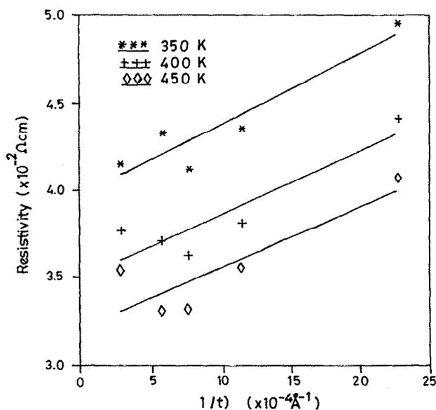
FIG. 4. Film resistivity vs reciprocal thickness plots of  $Ga_5Se_{20}Te_{75}$  films at three different temperatures showing linearity.
