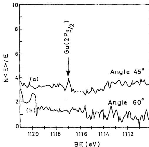
FIG. 8. XPS spectra relating to gallium [at (a) 45° and (b) 60°].
