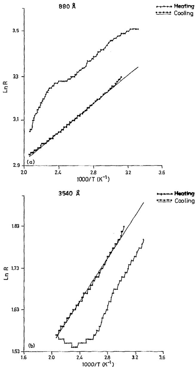
FIG. 3. Log resistance vs reciprocal temperature plots of the above films showing linearity during the cooling cycle.
