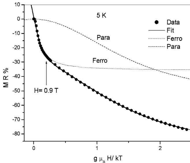
FIG. 4. The fit of MR as a function of  $x(=g\mu_B H/k_B T)$  at 5 K. The figure shows para- and ferromagnetic contributions separately.
