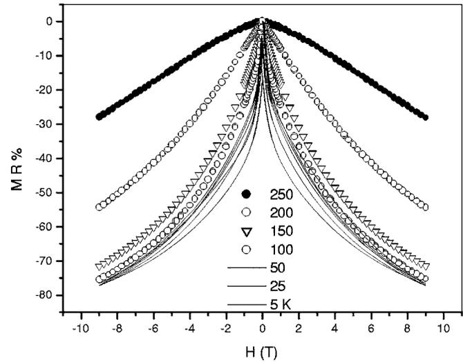
FIG. 3. MR as a function of an applied magnetic field  $H$ .
