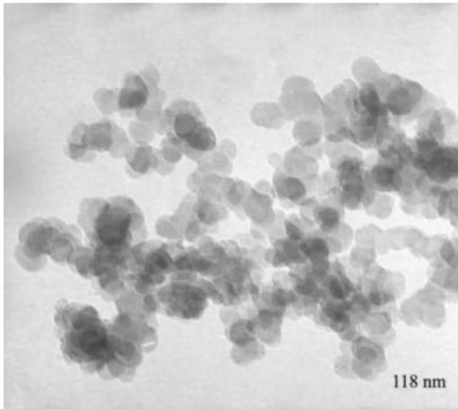
FIG. 1. TEM micrograph of the  $\text{Nd}_{0.7}\text{Sr}_{0.3}\text{MnO}_3$ .
