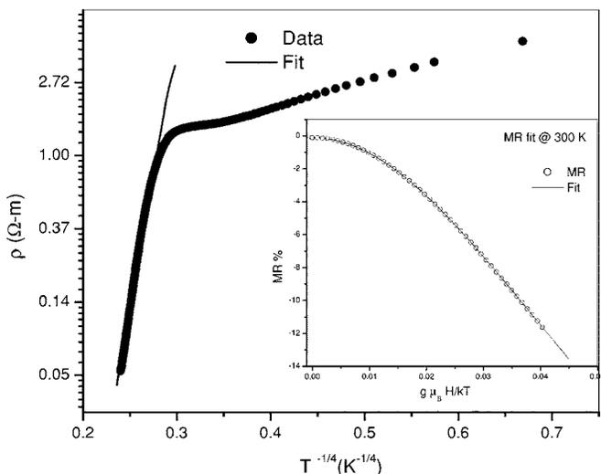
FIG. 2.  $\ln(\rho)$  as a function of  $T^{-1/4}$ . The fit yields a good fit over paramagnetic regime. The inset shows MR as a function of  $x(=g\mu_B H/k_B T)$  at 300 K. The solid line shows the fit to the data.
