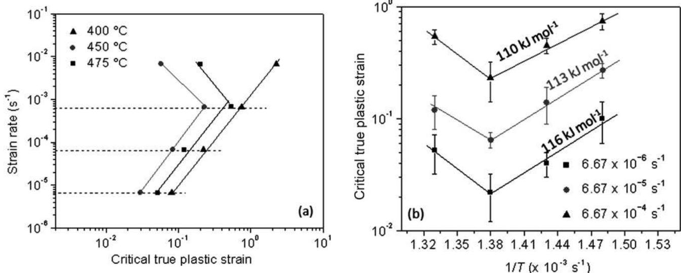
Fig. 8. Plots of (a)  $\ln(\text{strain rate})$  versus  $\ln(\epsilon_c)$  at different temperatures, and (b)  $\ln(\epsilon_c)$  versus  $1/T$  at different strain rates for Timetal 834. The activation energy determined by critical strain method is shown in (b).
