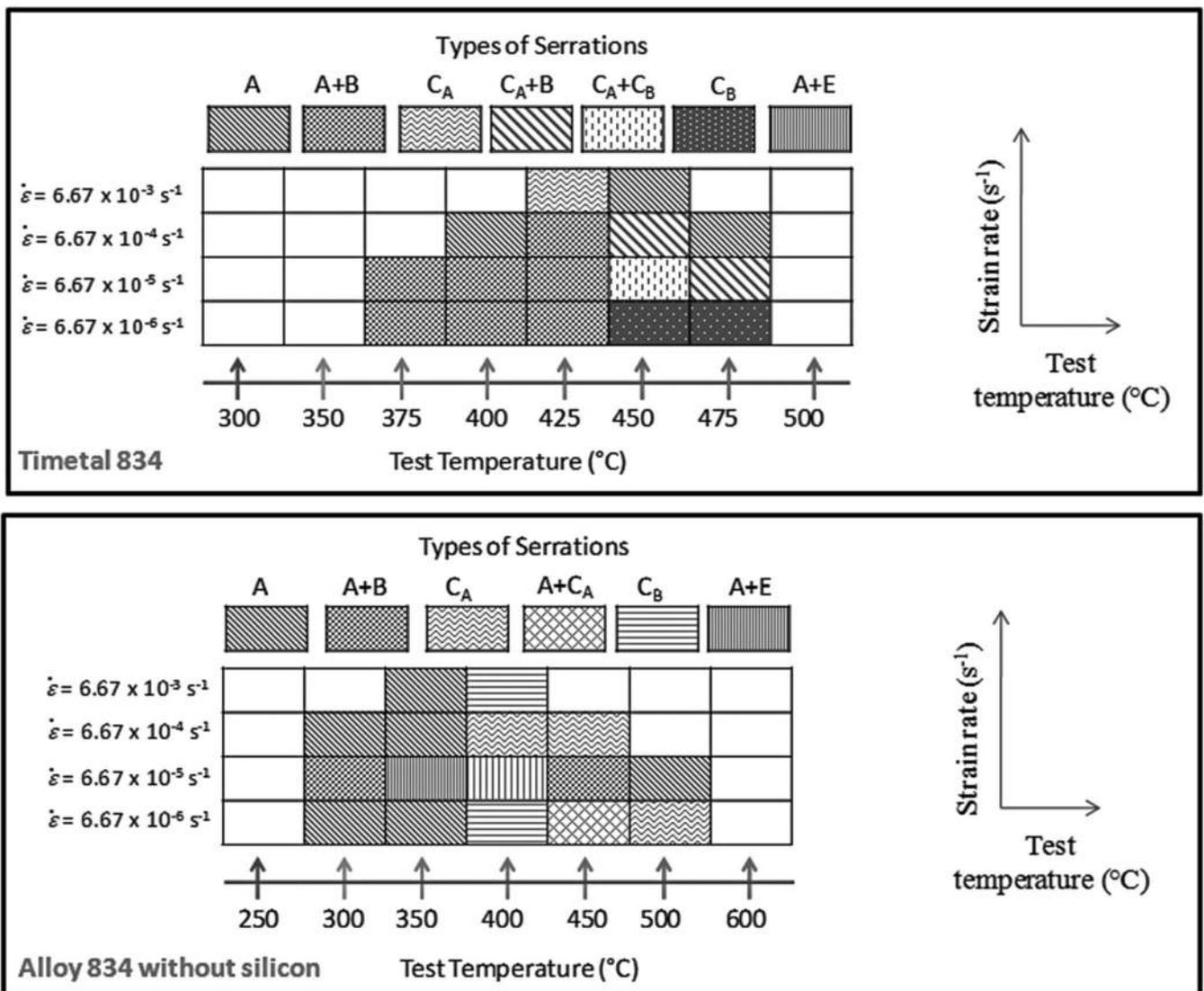
Fig. 3. The schematic classification of serrations as a function of temperature and strain rate for: (a) Timetal 834, and (b) alloy 834 without silicon.
