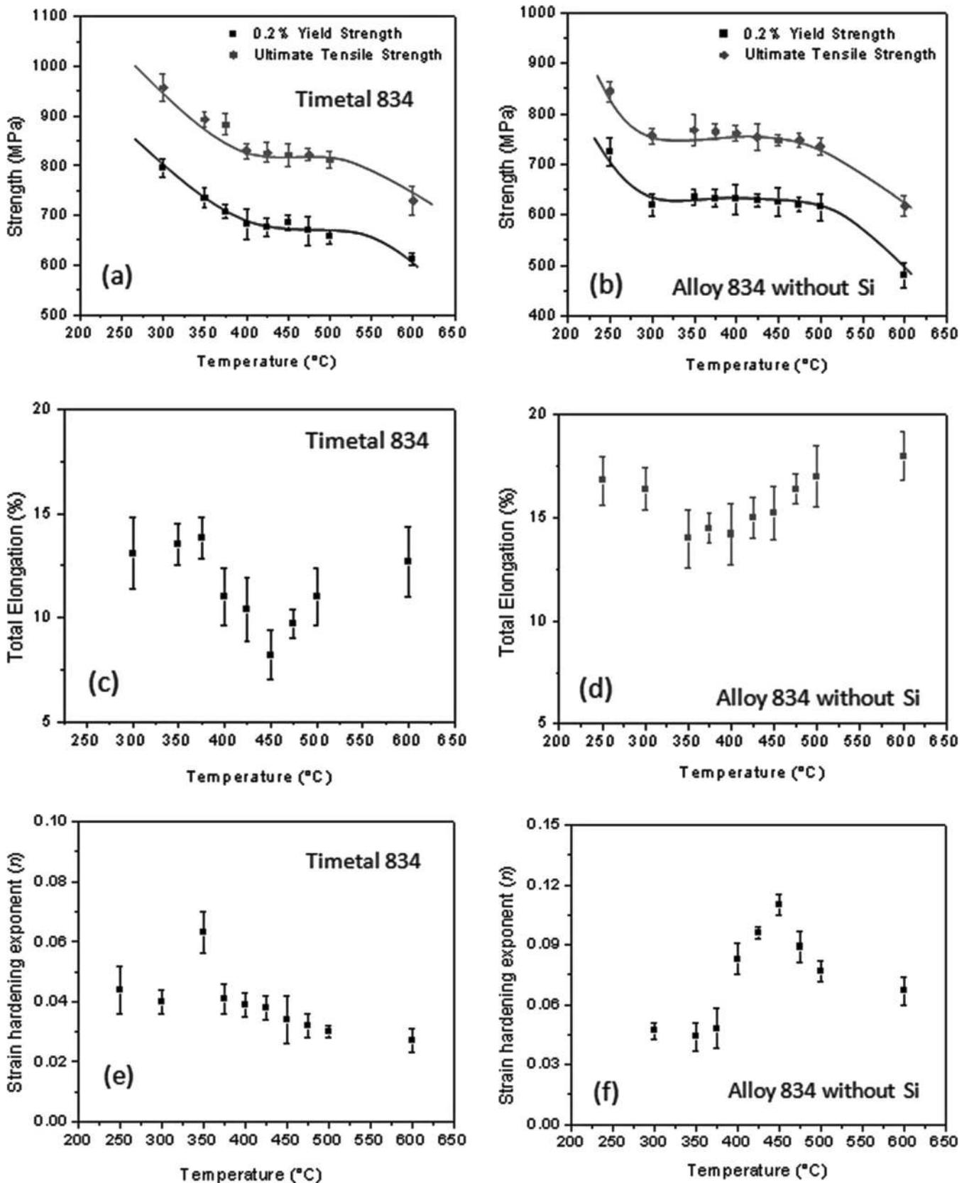
Fig. 4. Influence of temperature on: (a, b) 0.2% yield strength (MPa) and tensile strength (MPa), (c, d) % total elongation, and (e, f) strain hardening exponent of Timetal 834 (a, c, e) and alloy 834 without Si (b, d, f).
