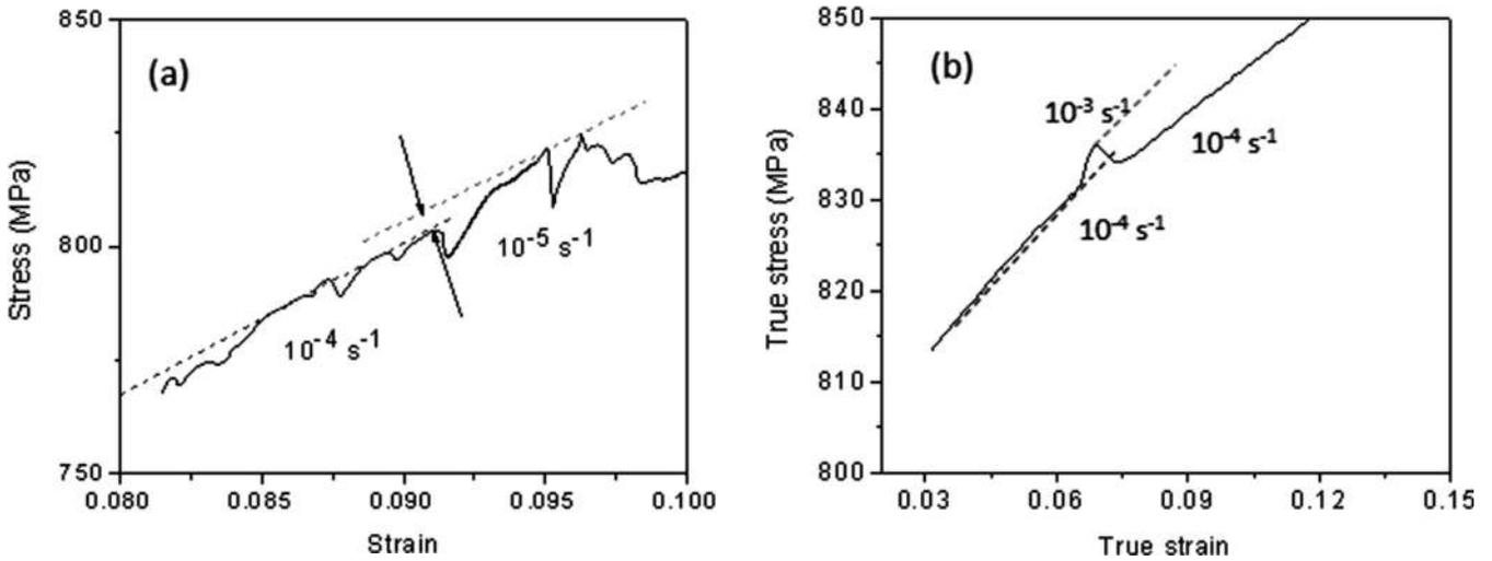
Fig. 5. Nature of transients during strain rate jump tests at: (a) 450 °C, serrated region, and (b) 300 °C, non-serrated region of Timetal 834.
