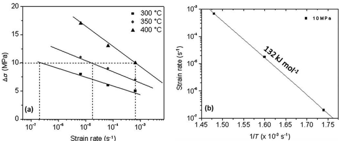
Fig. 12. Plots of (a)  $\Delta\sigma$  versus  $\ln$  (strain rate) at different temperatures, and (b)  $\ln$  (strain rate) versus  $1/T$  at  $\Delta\sigma = 10 \text{ MPa}$  in alloy 834. The activation energy determined by stress drop method in alloy 834 is shown in (b).
