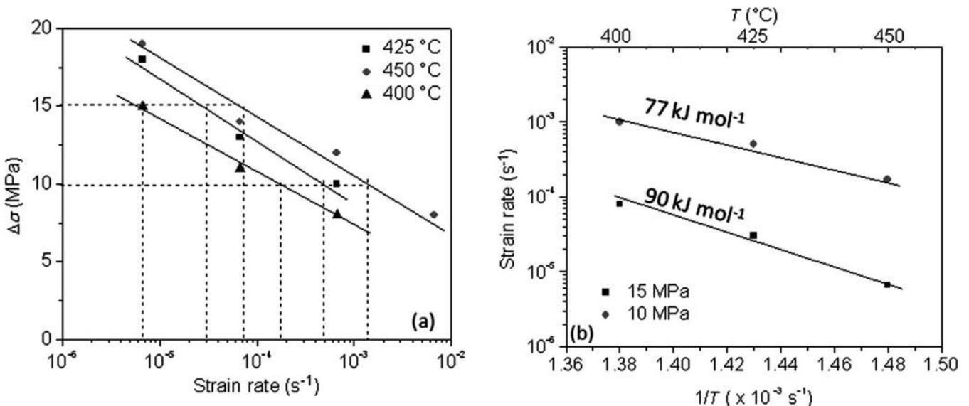
Fig. 10. Plots of (a)  $\Delta\sigma$  versus  $\ln(\text{strain rate})$  at different temperatures, and (b)  $\ln(\text{strain rate})$  versus  $1/T$  at different  $\Delta\sigma$  in Timetal 834. The activation energy determined by stress drop method is shown in (b).
