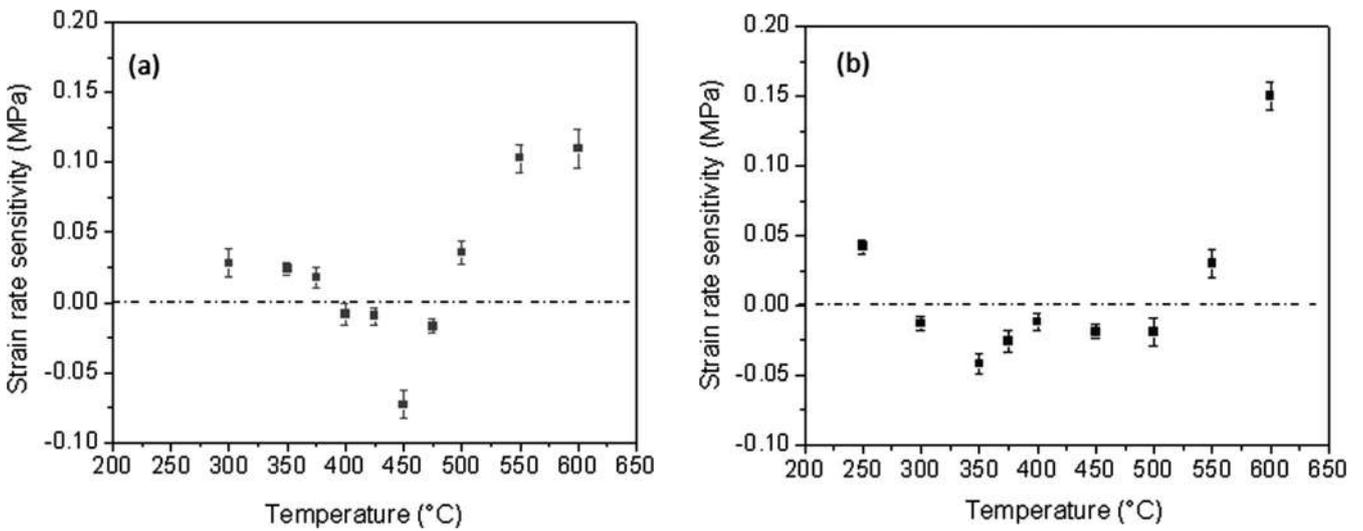
Fig. 6. Variation of strain rate sensitivity as a function of temperature of: (a) Timetal 834, and (b) alloy 834 without Si.
