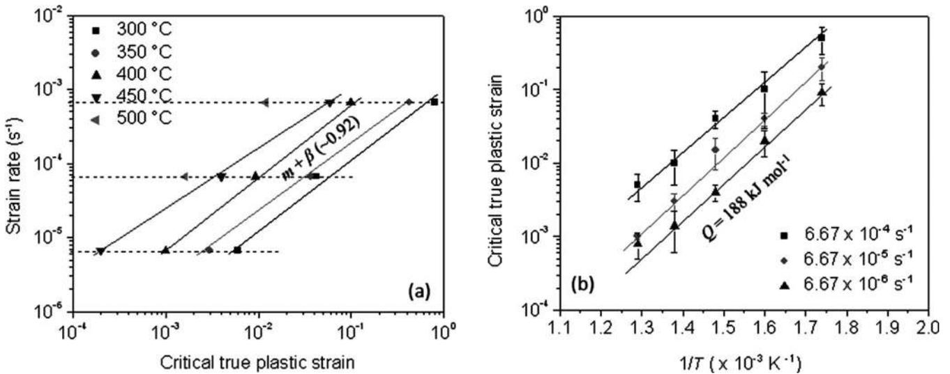
Fig. 11. Plots of (a) log (strain rate) vs log (critical plastic strain), and (b) log (critical plastic strain) vs. reciprocal temperature. The activation energy ( $\text{kJ mol}^{-1}$ ) determined by critical strain method in alloy 834 is shown in (b).
