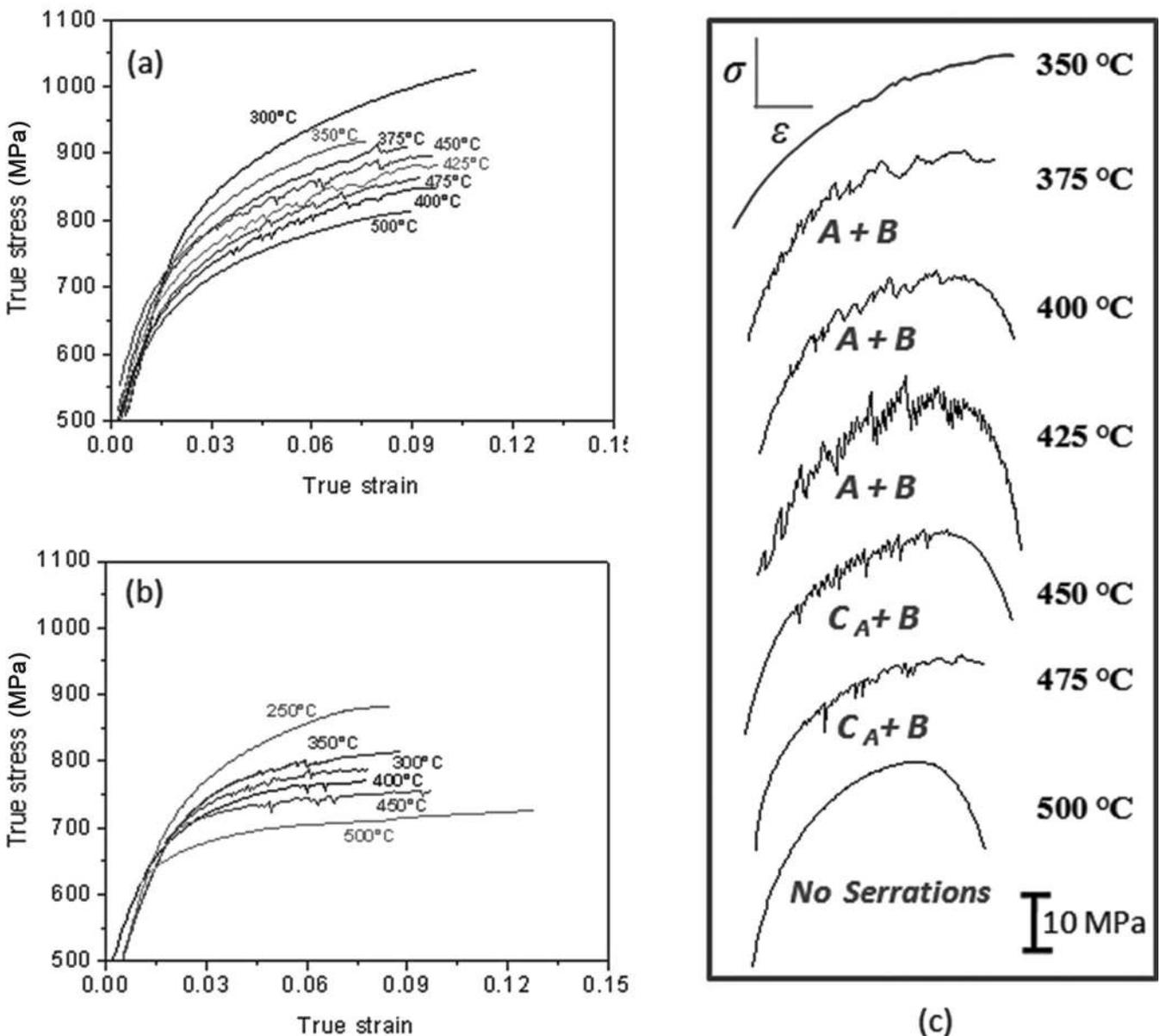
Fig. 2. Plastic region of true stress (MPa) – strain curves of: (a) Timetal 834, and (b) alloy 834 tested at a strain rate of  $6.67 \times 10^{-4} \text{ s}^{-1}$ . Various types of serrations manifested in Timetal 834 are shown in (c).
