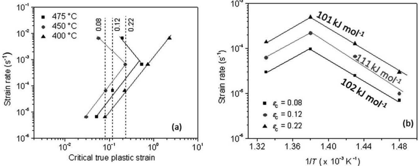
Fig. 9. Plots of (a)  $\ln(\text{strain rate})$  versus  $\ln(\epsilon_c)$  at different temperatures, and (b)  $\ln(\text{strain rate})$  versus  $1/T$  at different  $\epsilon_c$  in Timetal 834. The activation energy determined by intercept method is shown in (b).
