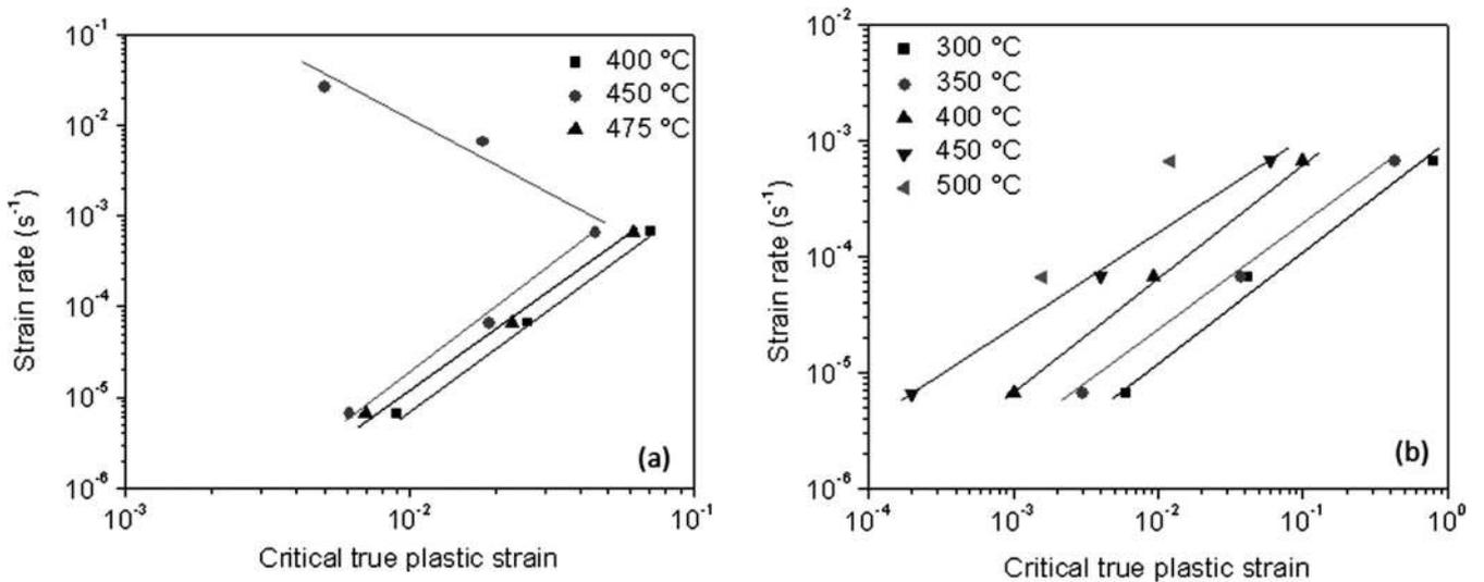
Fig. 7. Variation of critical true plastic strain with strain rate for the onset of serrations in: (a) Timetal 834, and (b) alloy 834.
