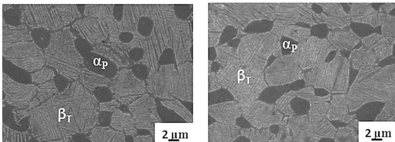
Fig. 1. SEM micrographs of (a) Timetal 834, and (b) alloy 834 without Si showing equiaxed primary  $\alpha$  and transformed  $\beta$  matrix.
