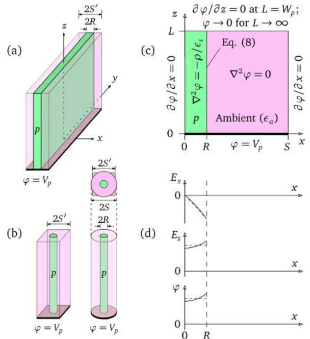
FIG. 3. (a) The simplified nanostructure of the NF array of Fig. 1(a). (b) The simplified nanostructure of the NW array of Fig. 1(b). (c) Equations and boundary conditions for analyzing the NF structure of (a). (d) Actual (solid lines) and approximate (dashed lines) distributions of the field and potential inside the NF of (a). (c) and (d) apply to the NW structure of (b) by replacing  $x$  by  $r$ , and Eq. (8) by Eq. (10).
