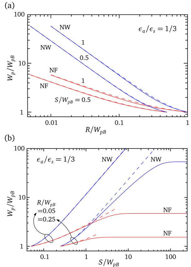
FIG. 4. (a) Depletion width as a function of NF/NW thickness with inter-film/wire separation as the parameter. (b) Depletion width as a function of inter-film/wire separation with NF/NW thickness as the parameter. Solid lines: Eq. (A4) for NF and Eq. (A5) for NW; dashed lines: closed form Eq. (13) for NF and Eq. (22) for NW.
