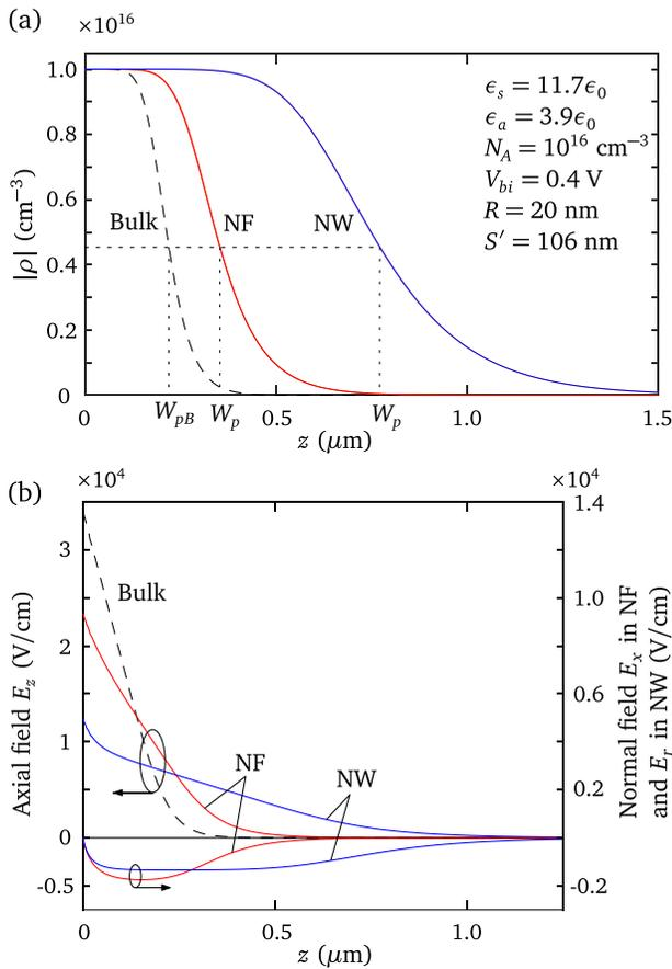
FIG. 2. Simulated equilibrium distributions of space-charge (a) and electric field (b) in Schottky junctions realized in bulk silicon, and in arrays of silicon NFs/NWs in  $\text{SiO}_2$  ambient.
