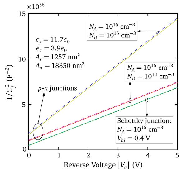
FIG. 7. The small-signal reverse bias capacitance-voltage characteristics of Schottky and  $p$ - $n$  junctions realized in arrays of silicon NWs in  $\text{SiO}_2$  ambient. Solid lines are numerical simulations of actual structures, and dashed lines are analytical calculations as per Effective Medium Theory.
