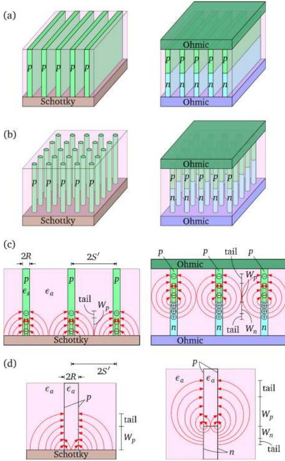
FIG. 1. Schottky and  $p$ - $n$  junctions in an array of nanofilms (a) and nanowires (b). The cross-sections of junctions in nanofilm and nanowire arrays are identical; (c) shows these and the field lines. A nanotube array appears like (b), except that the wires are hollow, and has the field lines shown in (d).
