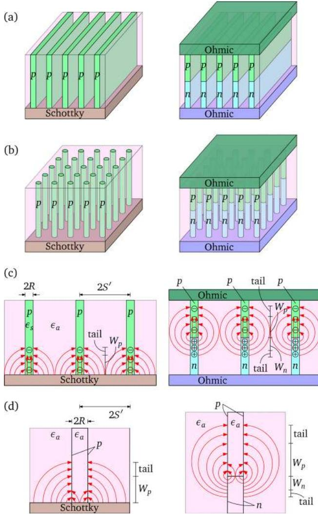
FIG. 1. Schottky and  $p$ - $n$  junctions in an array of nanofilms (a) and nanowires (b). The cross-sections of junctions in nanofilm and nanowire arrays are identical; (c) shows these and the field lines. A nanotube array appears like (b), except that the tubes are hollow, and has the field lines shown in (d). Reproduced with permission from J. Appl. Phys. **119**, 024507 (2016). Copyright 2016 AIP Publishing LLC.
