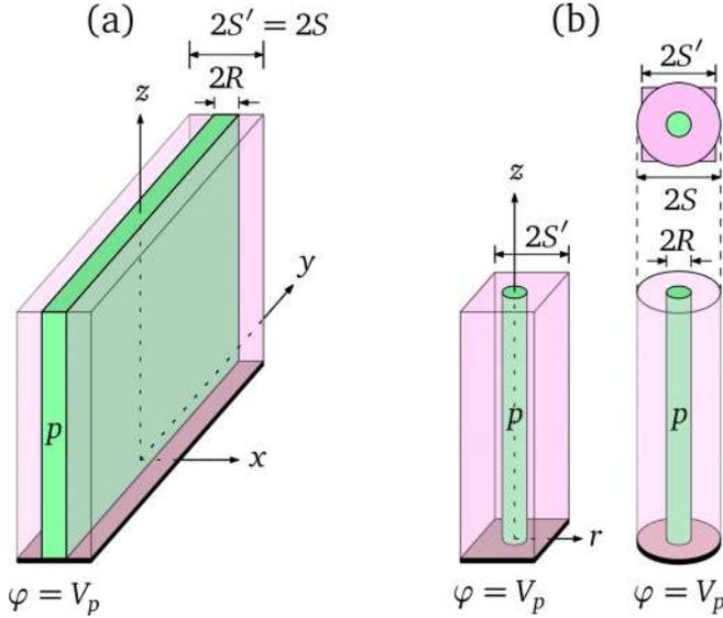
FIG. 2. (a) The simplified nanostructure of the NF array of Fig. 1(a). (b) The simplified nanostructure of the NW array of Fig. 1(b).
