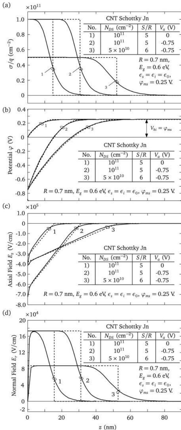
FIG. 5. Simulated distributions (solid lines) and our analytical models (dashed lines) in Schottky junctions realized in Carbon Nanotube arrays in air ambient. (a) Space-charge distributions; the box-like profiles are from the depletion width Eq. (19). (b) Potential distributions; model is Eq. (34). (c) Axial field distributions; model is Eq. (35). (d) Normal field distributions; model is Eq. (69). Note that the models are modified to suit the  $n$ -type Schottky junction with  $z > 0$ .
