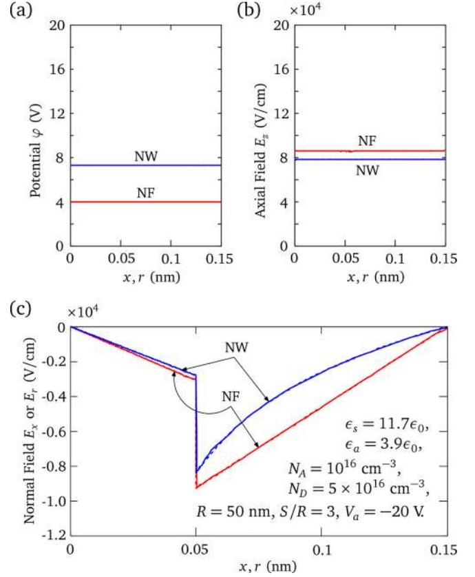
FIG. 4. Simulated distributions (solid lines) and our analytical models (dashed lines) as a function of  $x, r$  at  $z = 1 \mu\text{m}$  on the  $p$ -side of the junctions in Fig. 3. (a) Potential distributions; (b) axial field distributions; (c) normal field distributions. The analytical models employed are Eqs. (13), (19), (34), (35), (36), (37), (67), and (69).
