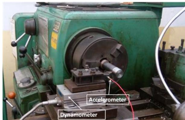
Fig. 2. Experimental setup to measure vibration
