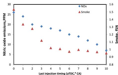
**Fig. 11. Variation of NO<sub>x</sub> and smoke emissions with last injection pulse timing with five pulses Injection.**
