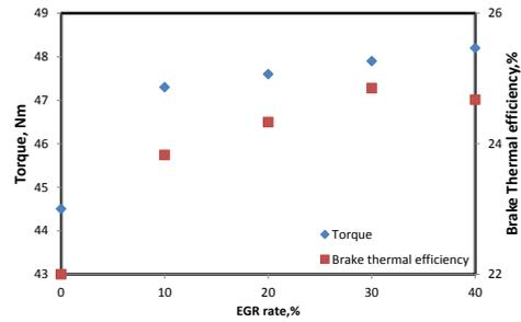
**Fig. 16. Variations of torque and Brake thermal efficiency with EGR rate with five pulses injection.**
