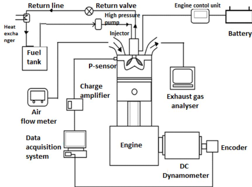
Fig. 1. Schematic of the experimental setup with instrumentation.
