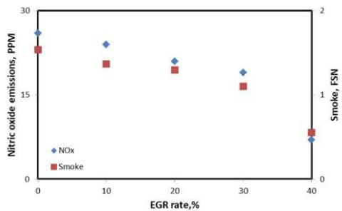
**Fig. 15. Variations of NOx and smoke emissions with EGR rate in five pulses injection.**
