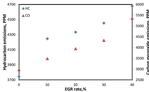
**Fig. 14. Variations of HC and CO emissions with EGR rate with five pulses injection.**
