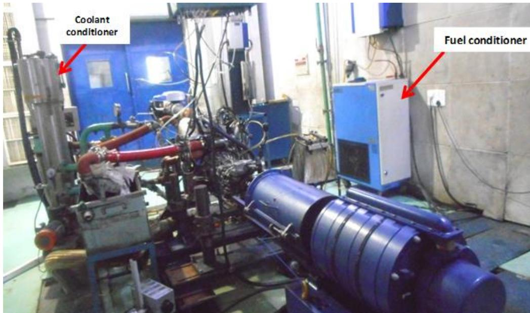
**Fig. 2. Test engine setup with instrumentation.**
