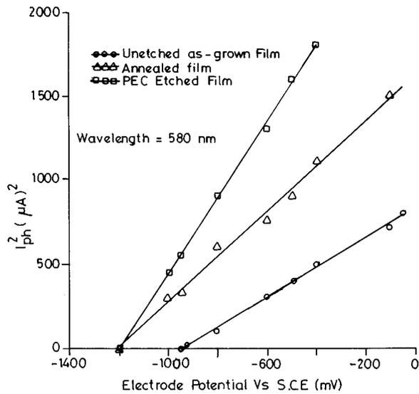
FIG. 7. A plot of  $I_{ph}^2$  vs Electrode potential for a monochromatic wavelength of 580 nm for the as-grown, annealed film and annealed-cum-PEC etched film.
