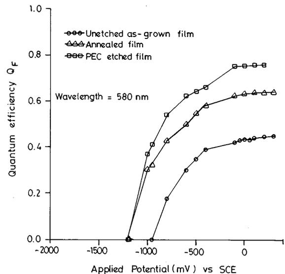
FIG. 12. A plot of quantum efficiency as function of applied potential for different surface treatments of  $n\text{-CdSe}_{0.6}\text{Te}_{0.4}/\text{polysulphide}$  PEC solar cell.
