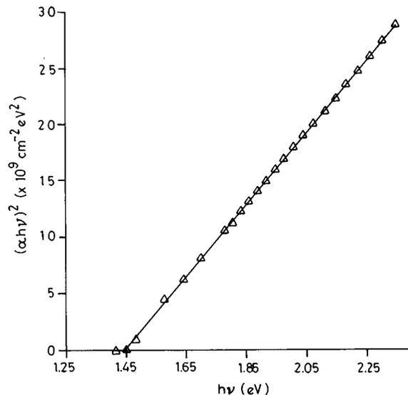
FIG. 2.  $(\alpha h\nu)^2$  vs  $h\nu$  plot of  $n$ -CdSe<sub>0.6</sub>Te<sub>0.4</sub> thin film of thickness 4000 Å.
