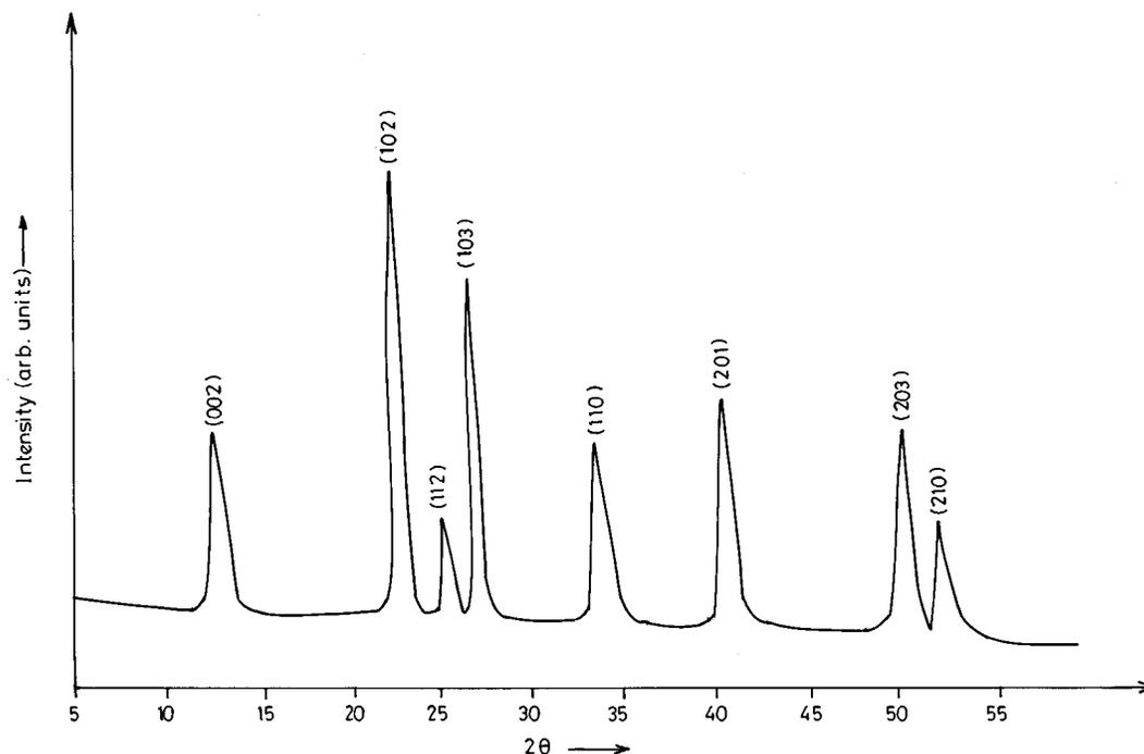
FIG. 1. An x-ray diffractogram of a typical  $n\text{-CdSe}_{0.6}\text{Te}_{0.4}$  thin film.
