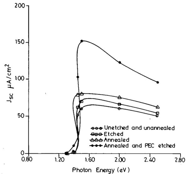
FIG. 9. A plot of  $J_{sc}$  as function of photon energy for  $n$ -CdSe<sub>0.6</sub>Te<sub>0.4</sub>/polysulphide PEC solar cell under various conditions.
