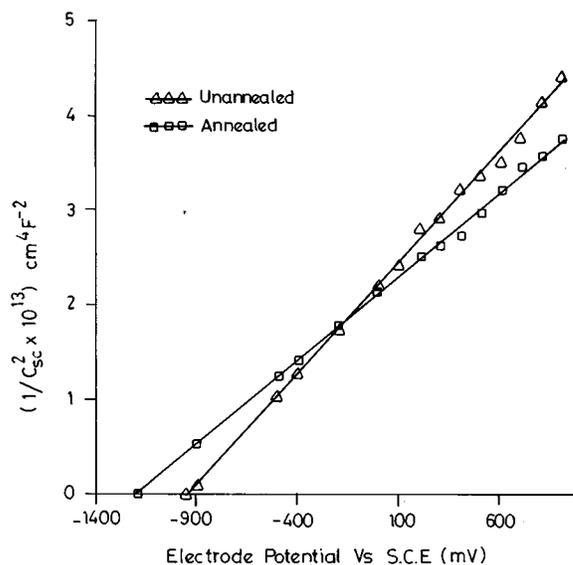
FIG. 3. Mott–Schottky plots for the annealed and unannealed  $n$ -CdSe<sub>0.6</sub>Te<sub>0.4</sub>/polysulphide system.
