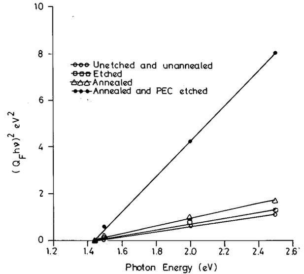
FIG. 11. A plot of  $(Q_F h\nu)^2$  as a function of photon energy for  $n\text{-CdSe}_{0.6}\text{Te}_{0.4}/\text{polysulphide}$  PEC solar cell.
