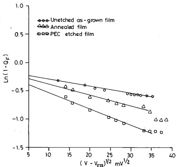
FIG. 13. A plot of  $\ln(1-Q_F)$  as a function of  $(V-V_{FB})^{1/2}$  using the Gärtner model.
