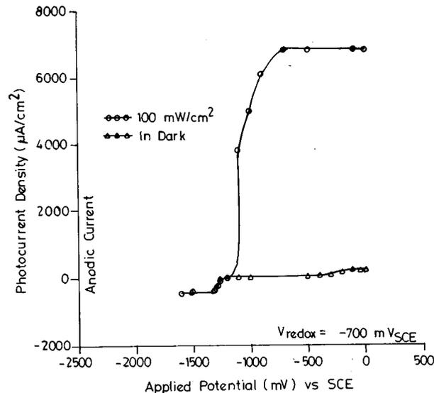
FIG. 6. Typical photocurrent density vs applied potential plot of  $n\text{-CdSe}_{0.6}\text{Te}_{0.4}$ /polysulphide PEC solar cell. Bottom curve signifies a feeble cathodic dark current.
