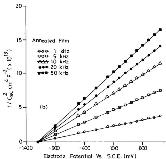
FIG. 5. (a) Mott-Schottky plots for the unannealed film used for  $n\text{-CdSe}_{0.6}\text{Te}_{0.4}$ /polysulphide system at frequencies of 1, 5, 10, 20, and 50 kHz. (b) Mott-Schottky plots for the annealed film used for  $n\text{-CdSe}_{0.6}\text{Te}_{0.4}$ /polysulphide system at frequencies of 1, 5, 10, 20, and 50 kHz.
