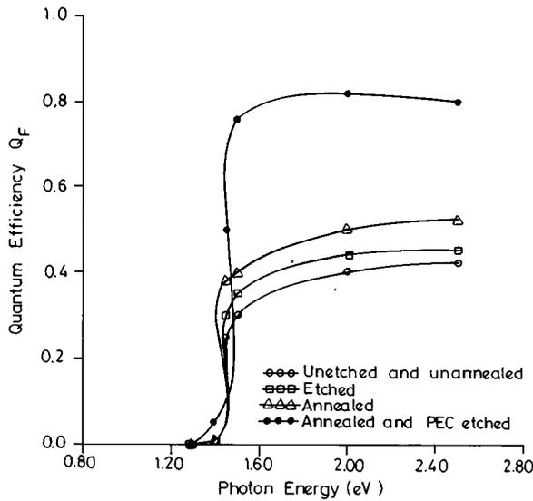
FIG. 10. A plot of quantum efficiency as function of photon energy for  $n\text{-CdSe}_{0.6}\text{Te}_{0.4}/\text{polysulphide}$  PEC solar cell.
