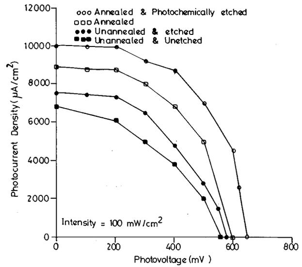
FIG. 8. Plot of power output characteristics for a typical  $n$ -CdSe<sub>0.6</sub>Te<sub>0.4</sub>/polysulphide PEC solar cell.
