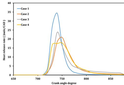
**Figure 11.** Comparison of heat release rate for various cases of SP and FI location
