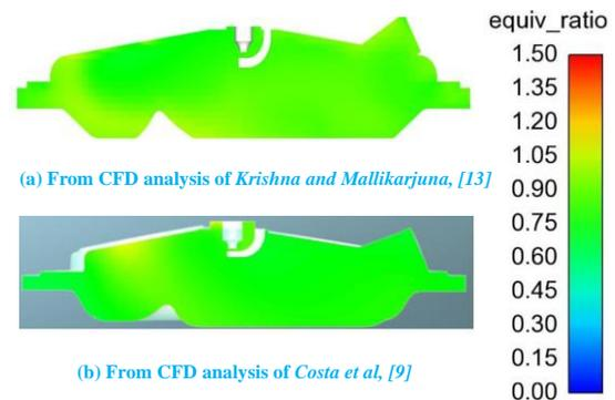
**Figure 4.** Comparison of ER distribution on central plane at spark timing
