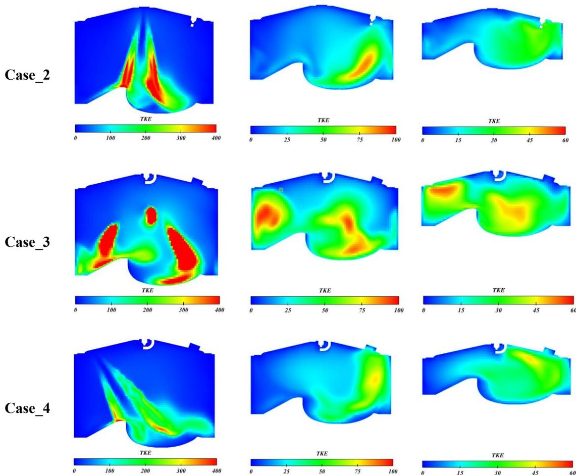
**Figure 5.** Comparison of TKE on the central plane at various CADs
