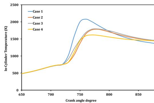
**Figure 10.** Comparison of in-cylinder temperature for various cases of SP and FI location
