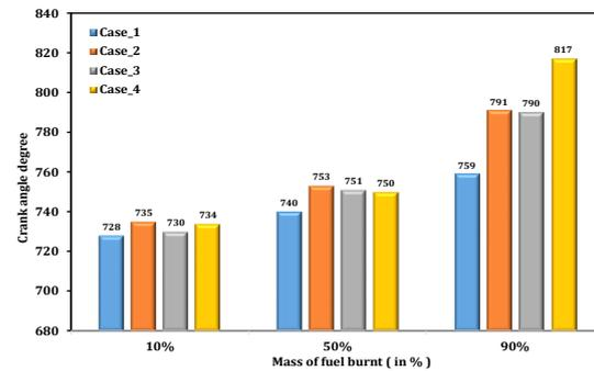
**Figure 12.** Comparison of mass fuel burnt for various cases of SP and FI location
