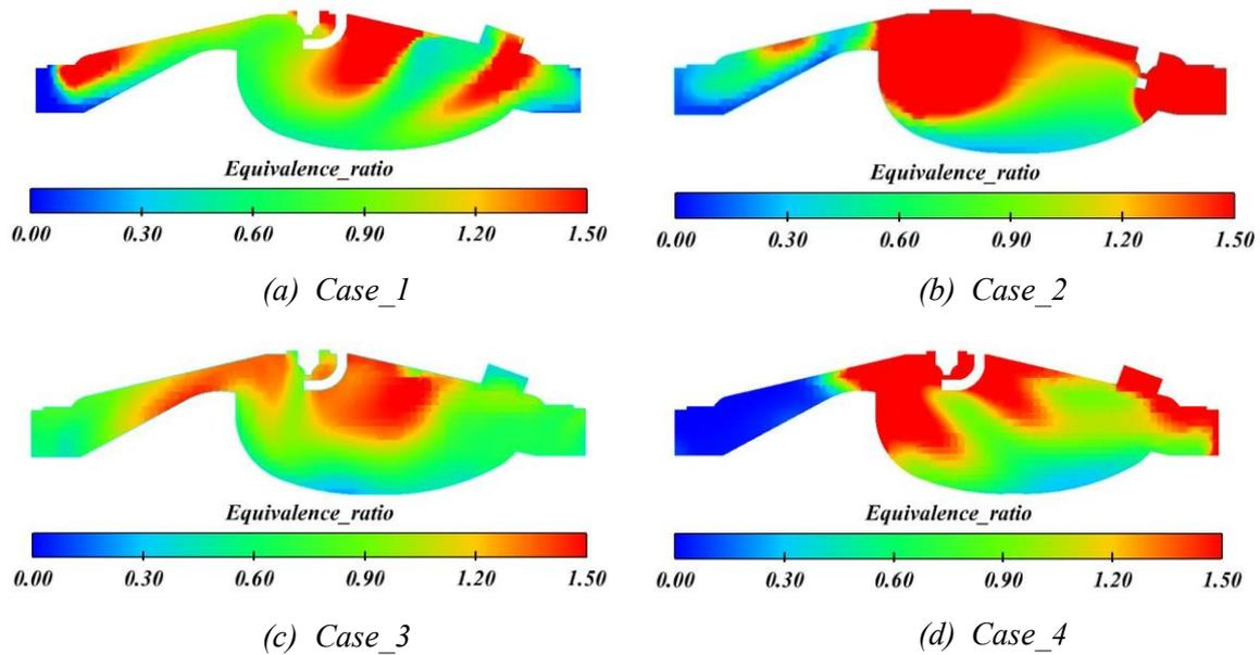
**Figure 6.** Comparison of ER distribution on the central plane at the spark timing
