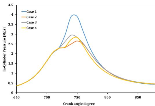
**Figure 9.** Comparison of in-cylinder pressure for various cases of SP and FI location
