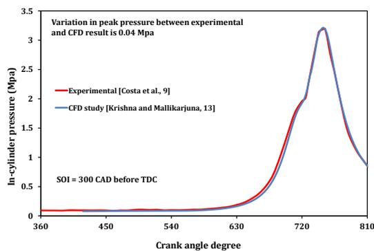
**Figure 3.** Comparison of in-cylinder pressure with crank angle degree
