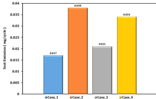
**Figure 15.** Comparison of soot emission at EVO for various cases of SP and FI location
