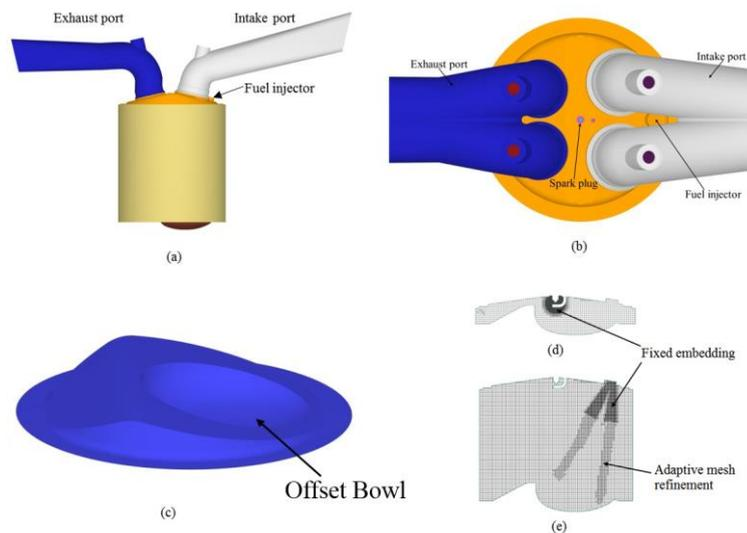
**Figure 2.** (a) Computational domain of the engine (b) Top view of engine (c) Piston with offset piston (d) Embedding at Spark (e) Adaptive mesh refinement at fuel injection
