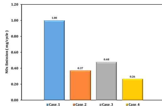
**Figure 14.** Comparison of NO<sub>x</sub> emission at EVO for various cases of SP and FI location
