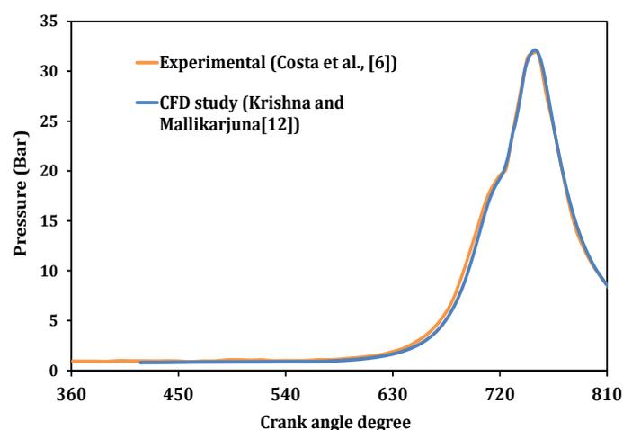
**Figure 3.** Comparison of in-cylinder pressure with crank angle degree
