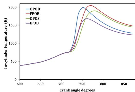
**Figure 8.** Comparison of in-cylinder temperature for various piston profiles
