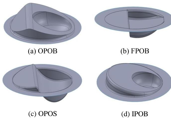
**Figure 2.** Various piston profiles used in the study
