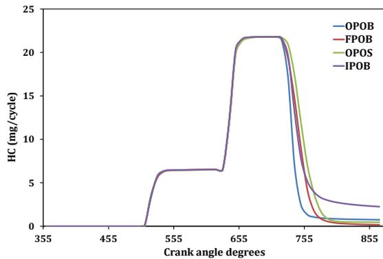
**Figure 12.** Comparison of HC formation for various piston profiles
