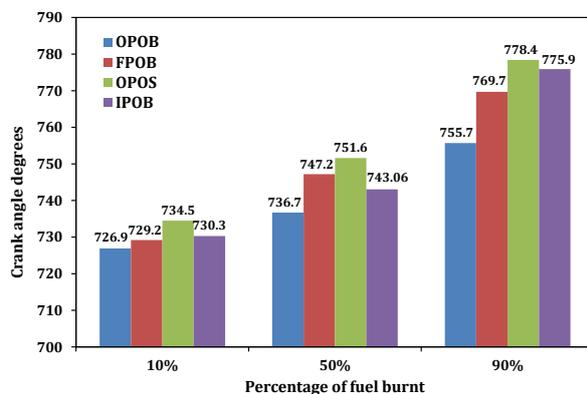
**Figure 10.** Comparison of percentage of fuel burnt for various piston profiles
