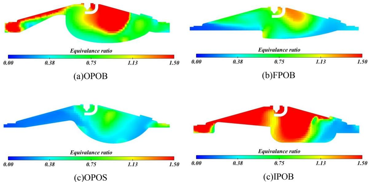
**Figure 6.** Comparison of ER for various piston profiles
