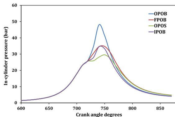
**Figure 7.** Comparison of in-cylinder pressure for various piston profiles
