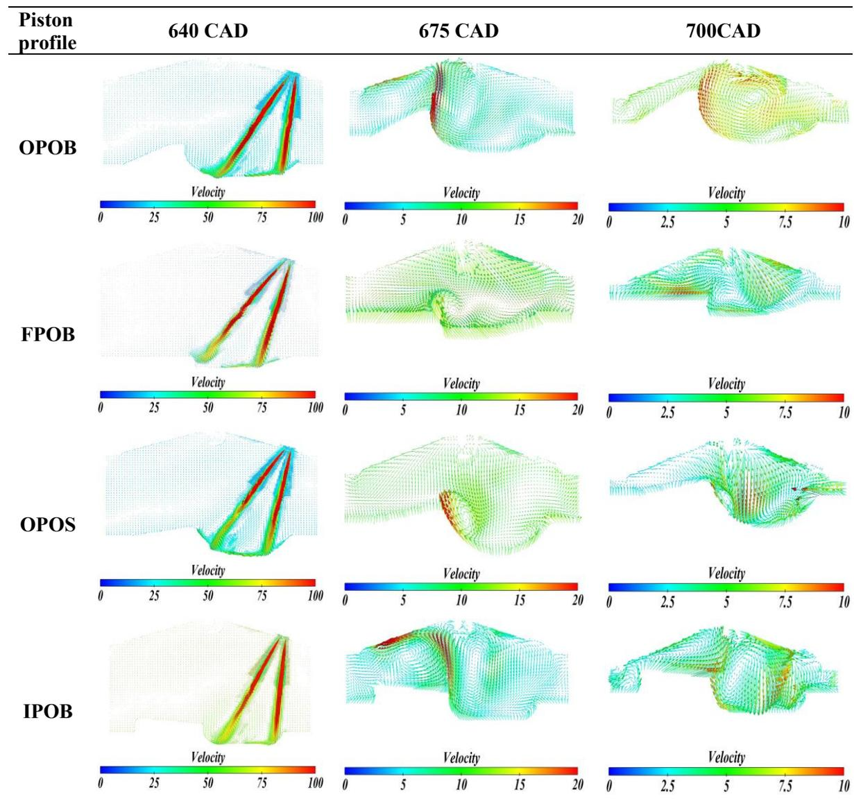
**Figure 5.** Comparison of in-cylinder flows for various piston profiles at various CAD
