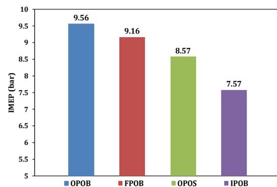
**Figure 11.** Comparison of IMEP for various piston profiles
