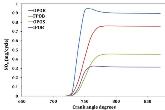
**Figure 13.** Comparison of NO<sub>x</sub> temperature for various piston profiles
