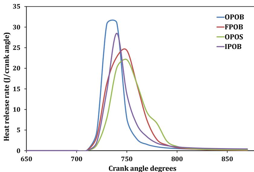
**Figure 9.** Comparison of heat release rate for various piston profiles
