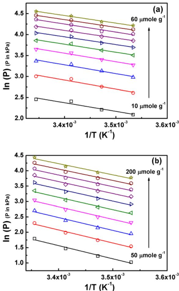
FIG. 8.  $\text{CO}_2$  adsorption isosteres (van't Hoff plot) of (a) MWNTs and (b) PEMWNTs with different adsorbed amount.
