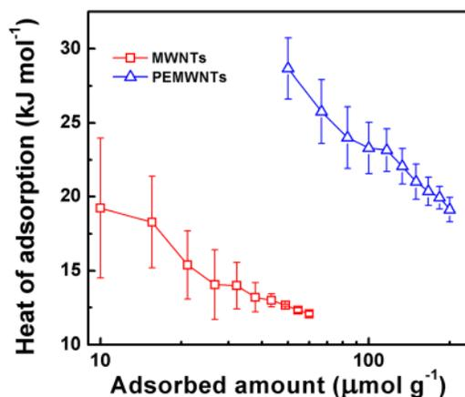
FIG. 9. Comparison of isosteric heats of adsorption of MWNTs and PEMWNTs as a function of adsorbed amount.
