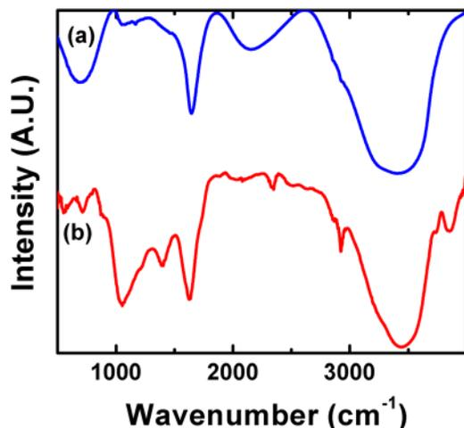
FIG. 3. FTIR spectra of (a) MWNTs and (b) PEMWNTs.
