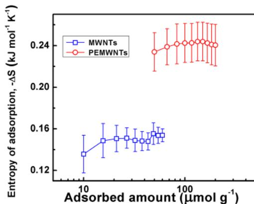
FIG. 10. Comparison of entropy change in adsorption of  $\text{CO}_2$  on MWNTs and PEMWNTs as a function of adsorbed amount.
