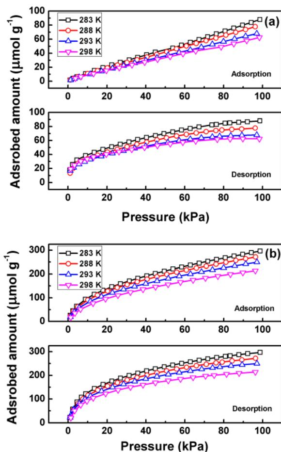
FIG. 5. CO<sub>2</sub> adsorption-desorption isotherms of (a) MWNTs and (b) PEMWNTs at multiple sample temperatures.
