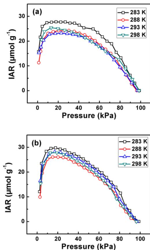
FIG. 6. Isothermal adsorbate retention of (a) MWNTs and (b) PEMWNTs as a function of equilibrium pressure.
