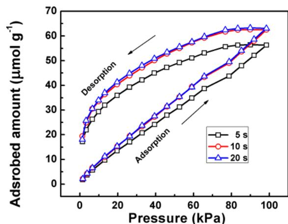
FIG. 4.  $\text{CO}_2$  adsorption-desorption isotherms of MWNTs at different equilibration intervals at 2% relative pressure tolerance and 200 Pa absolute pressure tolerance and 298 K sample temperature.
