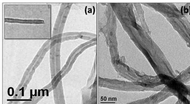
FIG. 2. Transmission electron micrograms of (a) MWNTs and (b) PEMWNTs.
