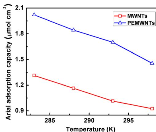
FIG. 7. Areal adsorption capacity of MWNTs and PEMWNTs at 283, 288, 293, and 298 K sample temperatures.
