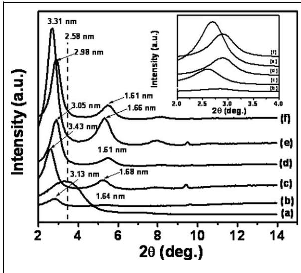
**Figure 4.** WAXD curves of PPO/PS-Cloisite 20A nanocomposites as a function of organoclay loading. (a) Cloisite 20A organoclay, (b) 2 wt%, (c) 4 wt%, (d) 6 wt%, (e) 8 wt% and (f) 10 wt%. Dashed vertical line shows the location of the organoclay d001 peak. WAXD: wide-angle x-ray diffraction; PPO: poly(phenylene oxide); PS: polystyrene.
