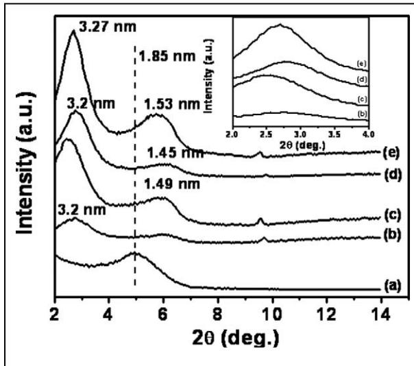
**Figure 2.** WAXD curves of PPO/PS-Cloisite 30B nanocomposites as a function of organoclay loading. (a) Cloisite 30B organoclay, (b) 2 wt%, (c) 4 wt%, (d) 6 wt%, (e) 8 wt% and (f) 10 wt%. Dashed vertical line shows the location of the organoclay d001 peak. WAXD: wide-angle x-ray diffraction; PPO: poly(phenylene oxide); PS: polystyrene.
