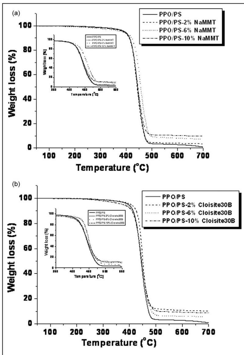
**Figure 6.** TGA thermographs; (a) PPO/PS-Na-MMT and (b) PPO/PS-Cloisite 30B. TGA: thermogravimetric analysis; PPO: poly(phenylene oxide); PS: polystyrene; Na-MMT: sodium montmorillonite.
