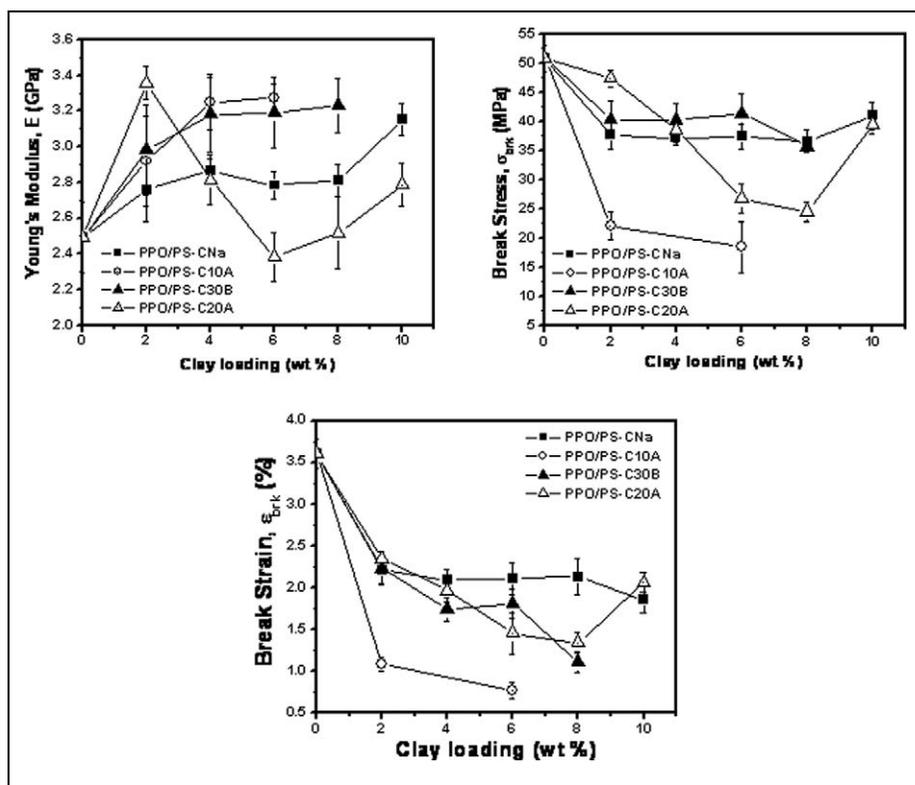
**Figure 7.** Variation in the mechanical properties of PPO/PS blend nanocomposite. PPO: poly(phenylene oxide); PS: polystyrene.
