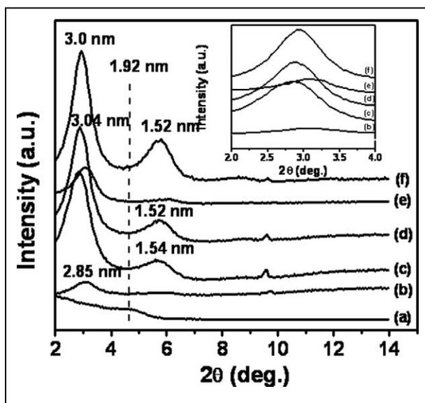
**Figure 3.** WAXD curves of PPO/PS-Cloisite 10A nanocomposites as a function of organoclay loading. (a) Cloisite 10A organoclay, (b) 2 wt%, (c) 4 wt%, (d) 6 wt%, (e) 8 wt% and (f) 10 wt%. Dashed vertical line shows the location of the organoclay d001 peak. Data for systems (a) to (c) are reproduced from Wiley, 2008.<sup>31</sup> WAXD: wide-angle x-ray diffraction; PPO: poly(phenylene oxide); PS: polystyrene.
