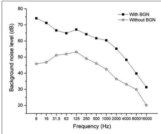
**Figure 1.** Noise spectrum with and without operation of ceiling fans.
