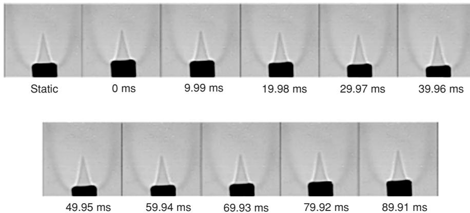
**Figure 5:** Instantaneous shadowgraphs of flames from static burner and burner vibrating with frequency 10 Hz and amplitude 1 mm ( $\Phi = 0.76$ ).
