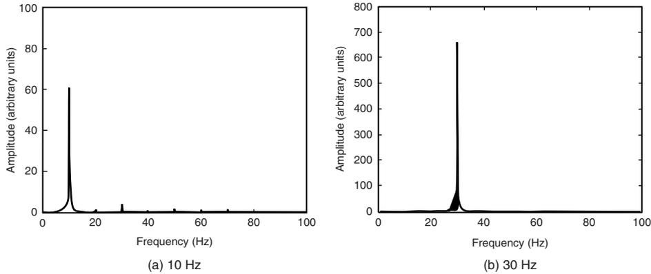
**Figure 2:** Acceleration spectra for exciter vibrations for 1 mm amplitude.
