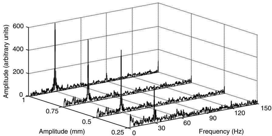
**Figure 10:** Spectra of flame height oscillations for 1 mm amplitude.
