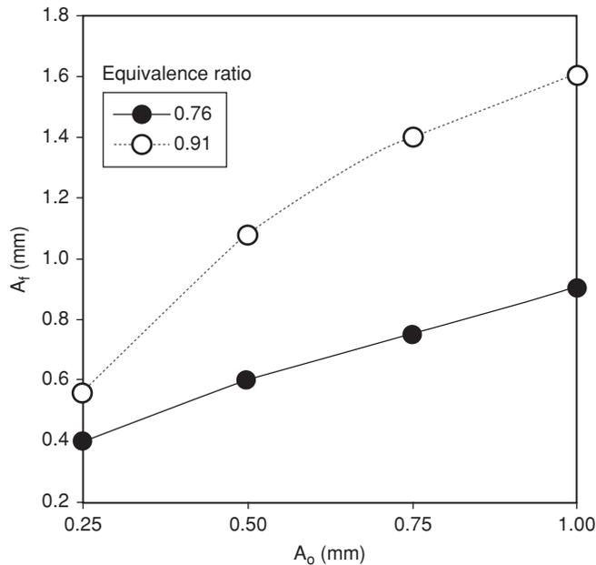
**Figure 9:** Amplitude of flame height oscillations for various equivalence ratios, at a frequency of 30 Hz.
