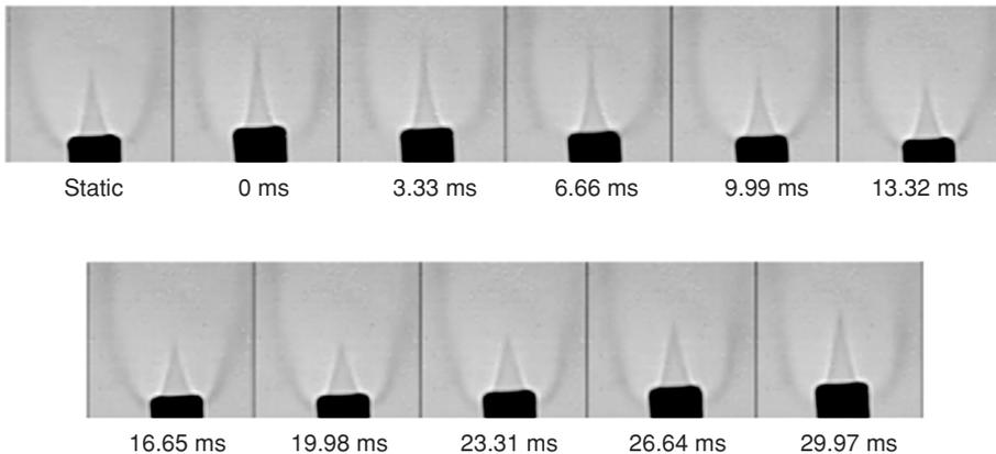
**Figure 7:** Instantaneous shadowgraphs of flames from static burner and burner vibrating with frequency 30 Hz and amplitude 1 mm ( $\Phi = 0.91$ ).
