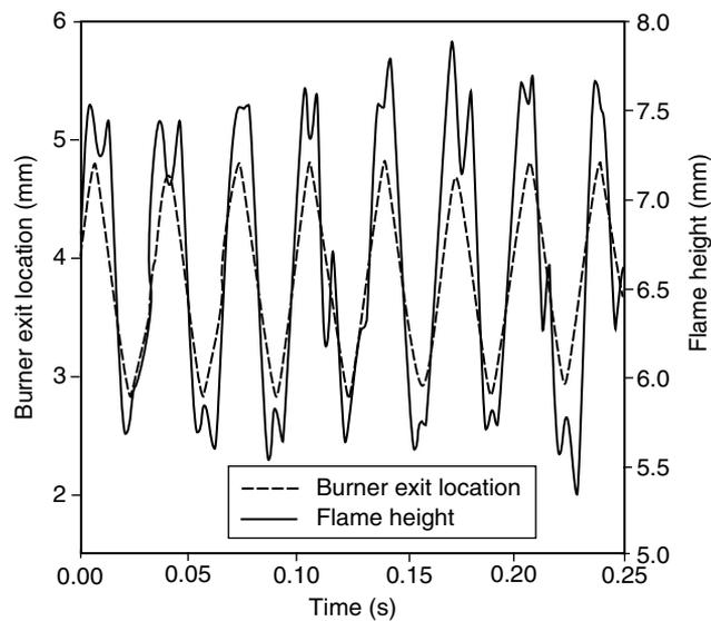
**Figure 11:** Time history of flame height oscillation and burner vibration for 30 Hz frequency and 1 mm amplitude.
