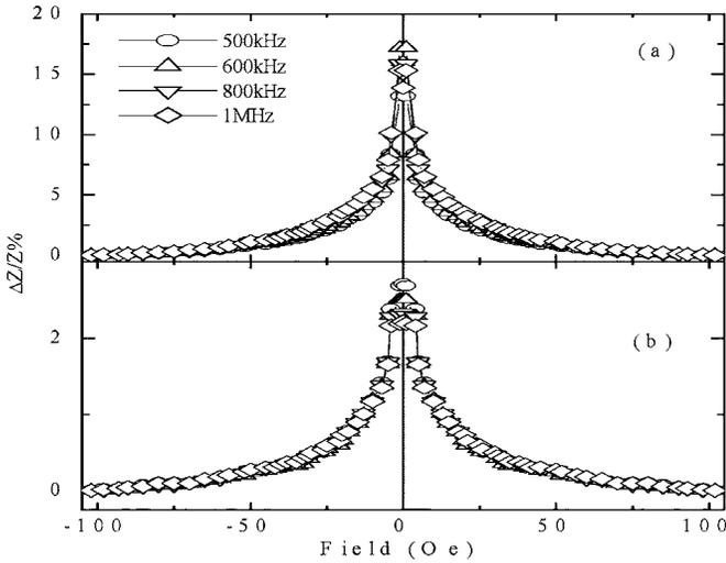
FIG. 1. MI of as cast  $\text{Co}_{68}\text{Fe}_5\text{Si}_{12}\text{B}_{15}$  ribbons of (a) 5 cm and (b) 1 cm length, respectively, measured at different frequencies.
