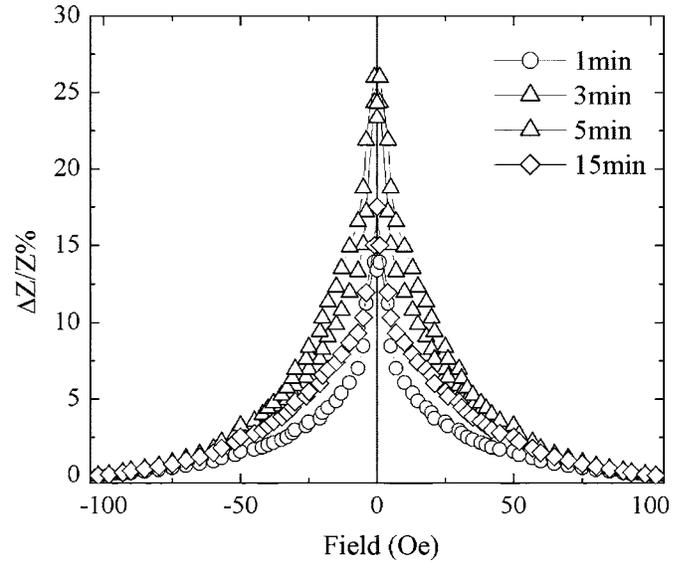
FIG. 3. MI at 800 kHz for Joule-annealed  $\text{Co}_{68}\text{Fe}_5\text{Si}_{12}\text{B}_{15}$  ribbons employing a 500 mA current.
