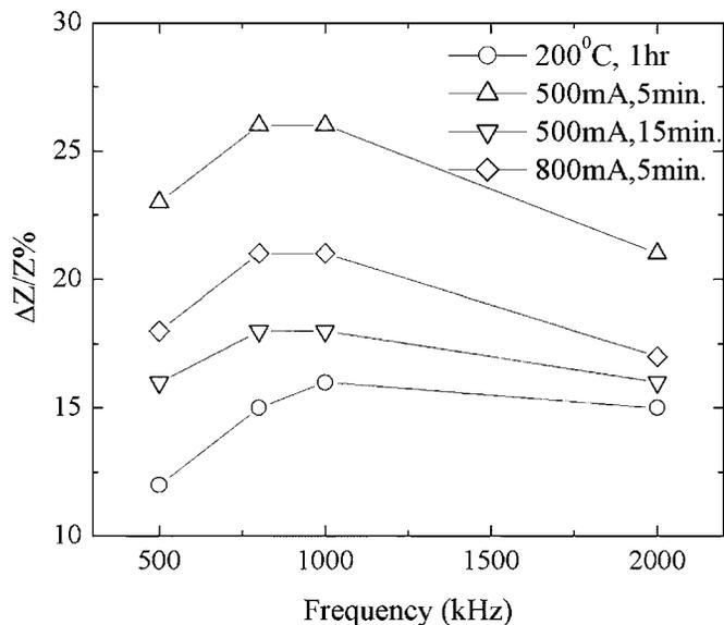
FIG. 5. Maximum MI of  $\text{Co}_{68}\text{Fe}_5\text{Si}_{12}\text{B}_{15}$  ribbons vs frequency for different annealing conditions.
