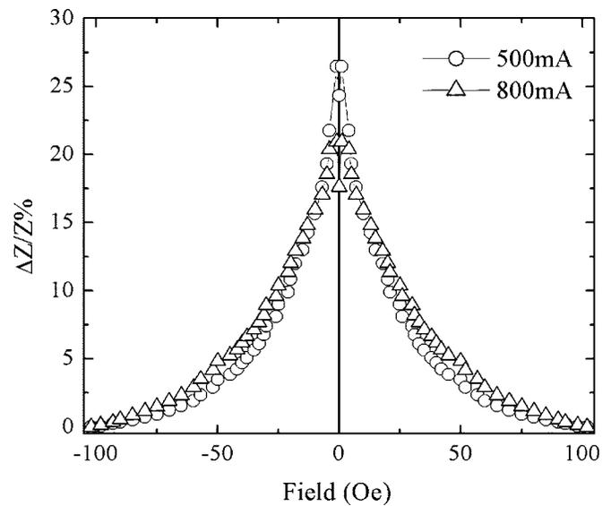
FIG. 4. MI at 800 kHz for Joule-annealed  $\text{Co}_{68}\text{Fe}_5\text{Si}_{12}\text{B}_{15}$  ribbons employing currents of 500 and 800 mA.
