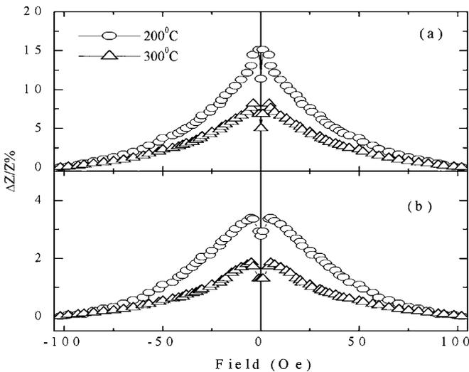
FIG. 2. MI of conventionally annealed  $\text{Co}_{68}\text{Fe}_5\text{Si}_{12}\text{B}_{15}$  ribbons of (a) 5 cm and (b) 1 cm long, at 800 kHz.
