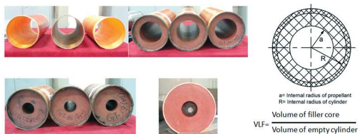
Figure 2. Typical photographs of empty and filled composite tubes.
