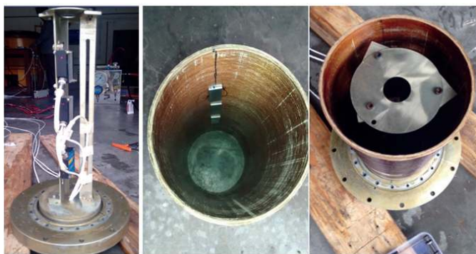
Figure 4. Photograph showing composite tube hardware assembly with NCDT: (a) NCDT on bracket, (b) Reflectors in tube, and (c) NCDT assembly with end plate.
