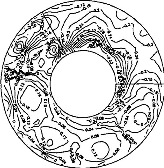
Fig. 12 Total pressure contours at rotor exit (without IGW,  $\phi = 0.45$ )
