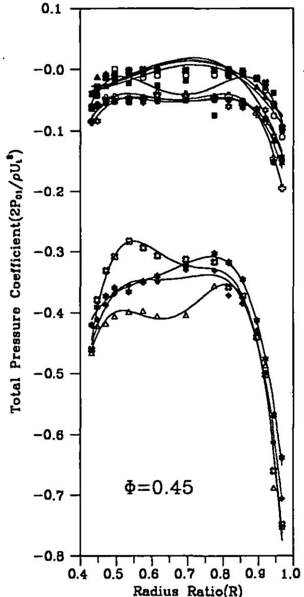
Fig. 5 Circumferentially averaged total pressure at rotor inlet (see Fig 4 for legend)
