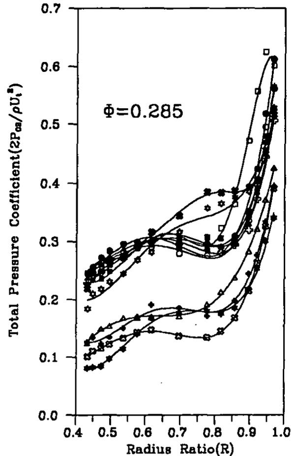
Fig. 8 Circumferentially averaged total pressure at rotor exit (see Fig 4 for legend)
