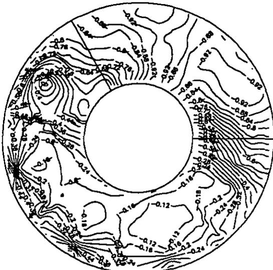
Fig. 6 Total pressure contours at rotor inlet (without IGV,  $\phi = 0.45$ )
