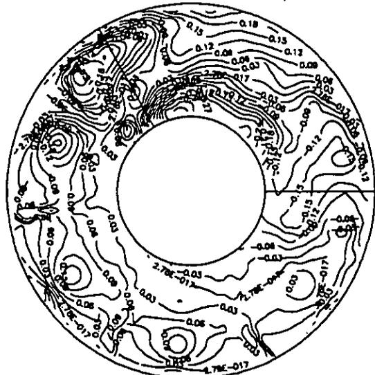
Fig. 17 Total pressure loss across stator ( $\gamma = -10^\circ$ ,  $\phi = 0.45$ )
