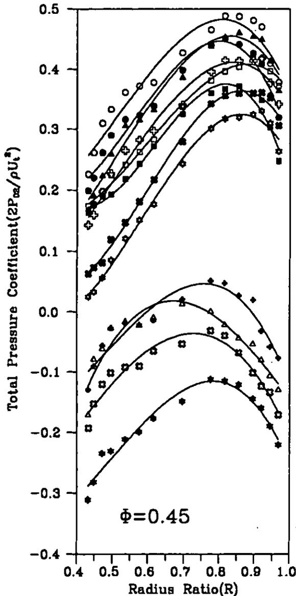
Fig. 9 Circumferentially averaged total pressure at rotor exit (see Fig 4 for legend)
