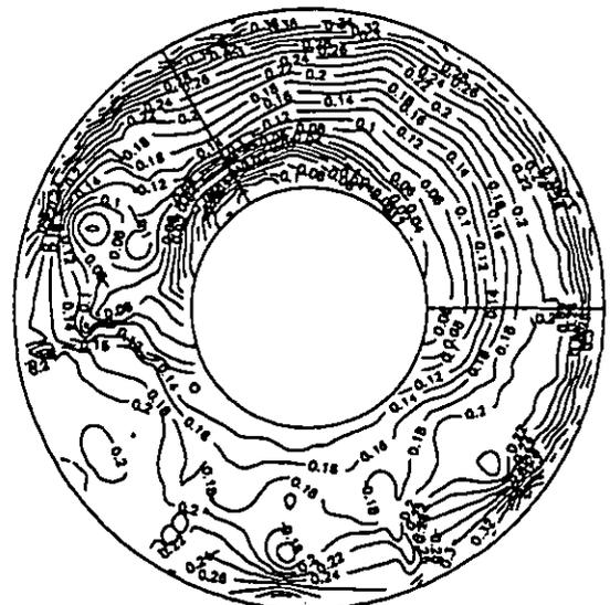
Fig. 11 Total pressure contours at rotor exit ( $\gamma = 5^\circ$ ,  $\phi = 0.285$ )
