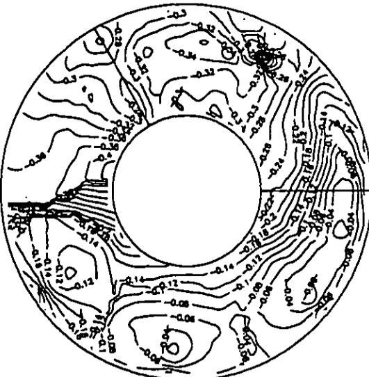
Fig. 15 Total pressure contours at stator exit ( $\gamma = 5^\circ$ ,  $\phi = 0.45$ )
