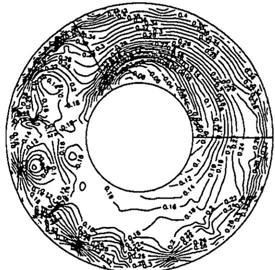
Fig. 10 Total pressure contours at rotor exit (without IGV,  $\phi = 0.285$ )
