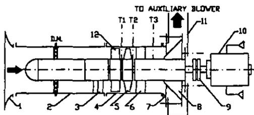
1. Inlet nozzle 2. Inlet duct 3. Radial supports 4. Impeller housing 5. Rotor 6. Stator 7. Discharge nozzle 8. Throttle cone 9. Coupling 10. D.C. Drive motor 11. Discharge casing 12. IG V T. Measuring planes D.M. Distortion mesh
