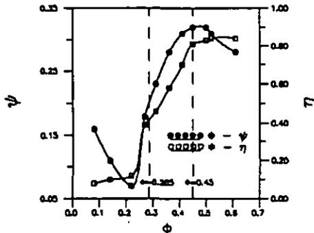
Fig. 3 Clean Inlet Operating Characteristics of the Fan
