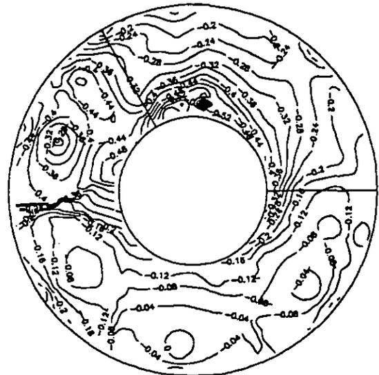
Fig. 13 Total pressure contours at rotor exit ( $\gamma = 5^\circ$ ,  $\phi = 0.45$ )
