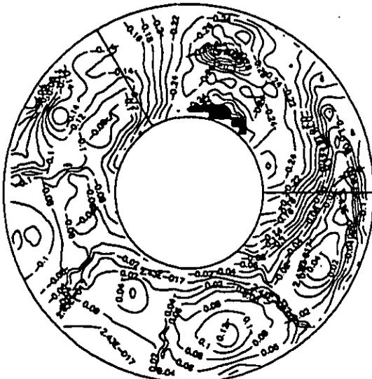
Fig. 14 Total pressure contours at stator exit (without IGW,  $\phi = 0.45$ )
