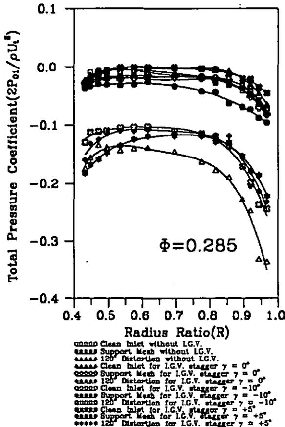
Fig. 4 Circumferentially averaged total pressure at rotor inlet
