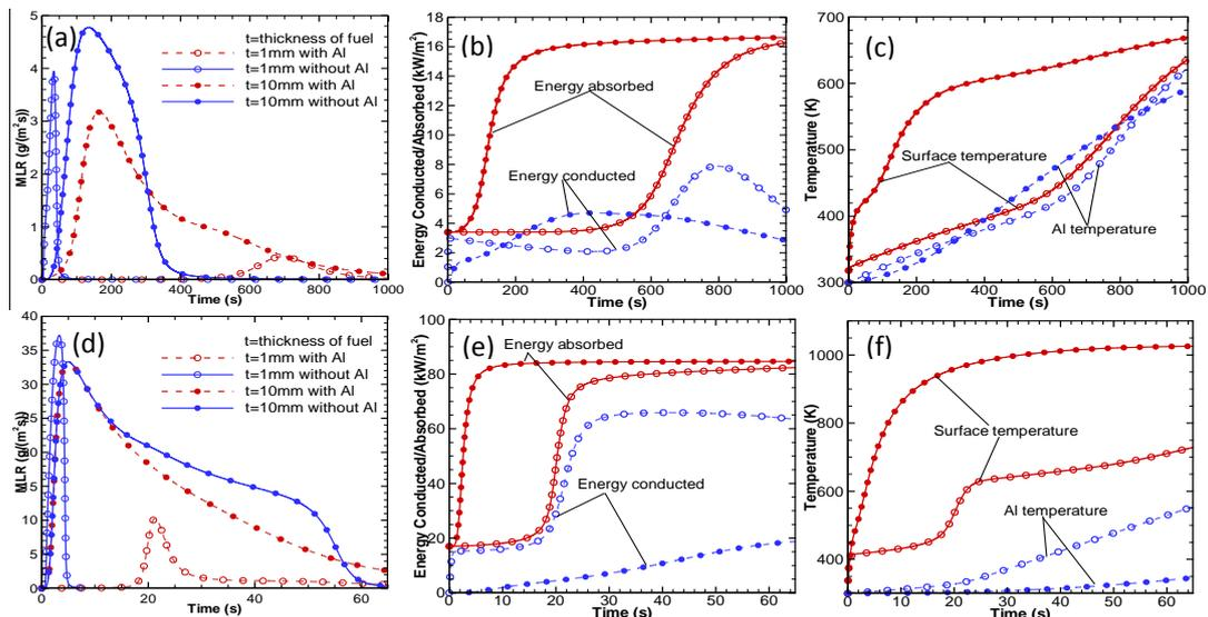
Fig. 4 Influence of thermal boundary condition on charring material pyrolysis (a),(b),(c) for 20 kW/m<sup>2</sup> and (d),(e),(f) for 100 kW/m<sup>2</sup>. Clear circles represent thin fuel (1mm) and solid circles represent thick fuel (10mm). (a) and (d) MLR comparison with and without Al block. (b) and (e) Energy absorbed (solid line) and conducted (dashed line) to Al block during pyrolysis. (c) and (f) surface (solid line) and Al block (dashed line) temperature variation.
