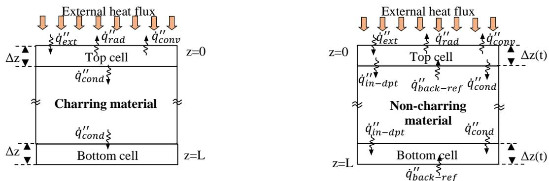
Fig. 1 Schematic of thermal boundary condition for charring and non-charring material.
