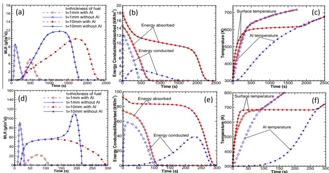
Fig. 5 Influence of thermal boundary condition on non-charring material pyrolysis (a),(b),(c) for  $20\text{ kW/m}^2$  and (d),(e),(f) for  $100\text{ kW/m}^2$ . Open circles represent thin fuel (1mm) and solid circles represent thick fuel (10mm). (a) and (d) MLR comparison with and without Al block. (b) and (e) Energy absorbed (solid line) and conducted (dashed line) to Al block during pyrolysis. (c) and (f) surface (solid line) and Al block (dashed line) temperature variation.
