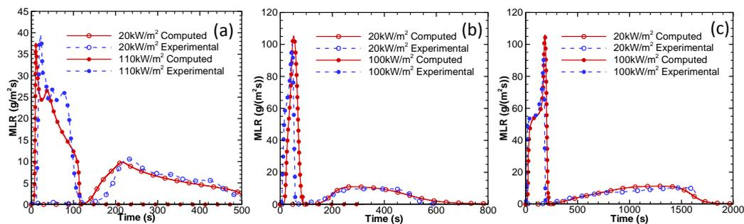
Fig. 2 Comparison between experimental [5] and numerical predictions. (a) 1.58 mm thick charring material (CPVC). (b) 3.18 mm thick non-charring material (PMMA). (c) 9.53 mm thick non-charring (PMMA) material.
