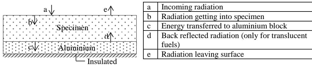
Fig. 3 Schematic of modified boundary condition.
