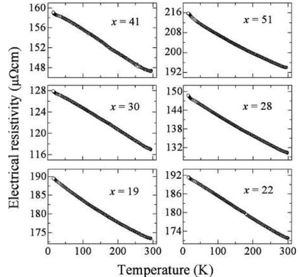
FIG. 5. Electrical resistivity of  $Tb_xFe_{100-x}$  films in the temperature range 13–300 K.
