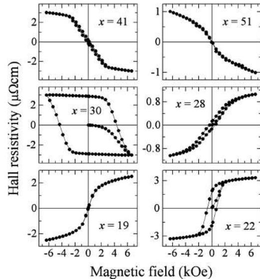
FIG. 3. HR of  $Tb_xFe_{100-x}$  films at room temperature.
