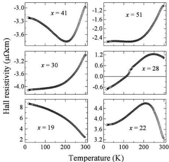
FIG. 6. HR of  $Tb_xFe_{100-x}$  films in the temperature range 13–300 K.
