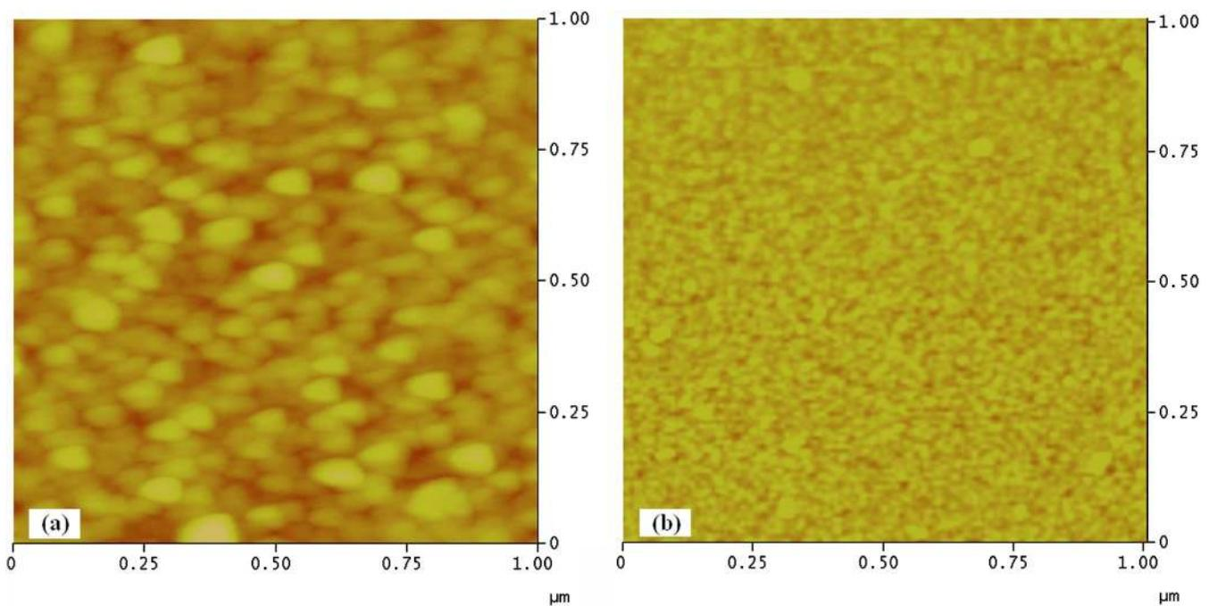
FIG. 2. (Color online) AFM images of  $Tb_xFe_{100-x}$  films of (a)  $x=9$  and (b)  $x=41$  contents.
