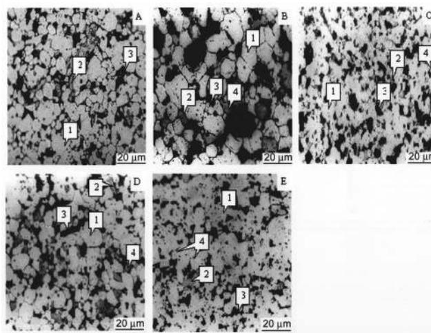
FIG. 6. Optical micrographs of sintered samples of (a) 36Nd-1.2B-Fe, (b) 36Nd-1.2B-1Al-Fe, (c) 36Nd-1.2B-1Cu-Fe, (d) 36Nd-1.2B-1Ga-Fe, and (e) 36Nd-1.2B-1Nb-Fe. The micrographs show the  $\varphi$  phase (1),  $\eta$  phase (2), Nd-rich phase (3), and a new phase with a high concentration of an additive element (4).
