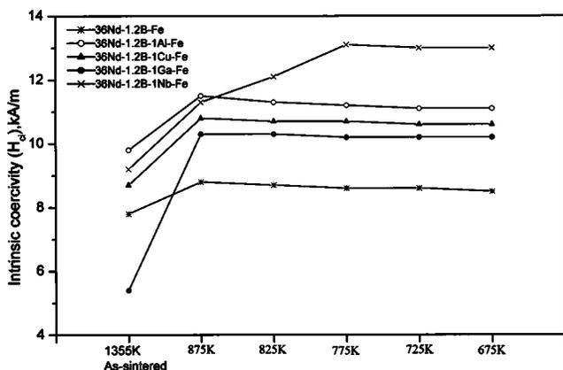
FIG. 3. Effect of heat treatment on the coercivity development in sintered samples of NdFeB with and without the addition of Al, Cu, Ga, and Nb.
