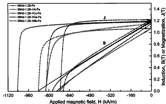
FIG. 2. Second quadrant hysteresis loop of sintered alloys, heat treated to achieve peak values of  $H_{ci}$ .
