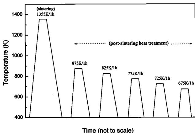
FIG. 1. Sintering and postsintering heat treatment schedule adopted for NdFeB samples.
