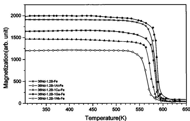
FIG. 4. Thermomagnetic plots of sintered NdFeB samples with and without additive elements, Al, Cu, Ga, and Nb.
