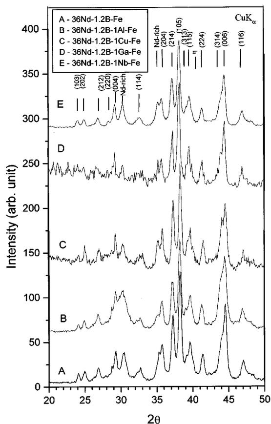
FIG. 5. X-ray diffraction patterns of sintered NdFeB magnet samples with and without additive elements, Al, Cu, Ga, and Nb. The patterns indicate the presence of three phases, viz. the  $\varphi$  phase, the  $\eta$  phase, and the Nd-rich phase.
