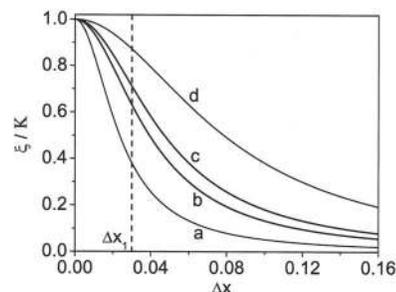
FIG. 7. The variation of the change in enhancement of the radiative rate with the detuning of the  $x$  parameter for microsphere diameters of (a)  $3 \mu\text{m}$ , (b)  $5 \mu\text{m}$ , (c)  $6 \mu\text{m}$ , and (d)  $10 \mu\text{m}$ .
