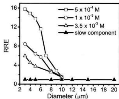
FIG. 6. The RRE ( $\xi$ ) plotted as a function of the diameter of the single PMMA microsphere for varying doping concentrations.
