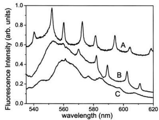
FIG. 4. Fluorescence spectra of Rhodamine 6G in  $\sim 2\text{-}\mu\text{m}$ -radius single PMMA microsphere as a function of concentration. The concentrations are (A) 5 mM, (B) 10 mM, and (C) 100 mM.
