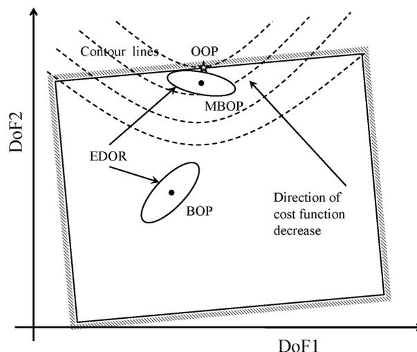
Fig. 1. Idea of back off operating point selection
