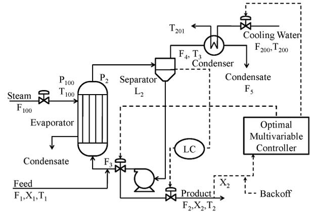
Fig. 2. Evaporator system
