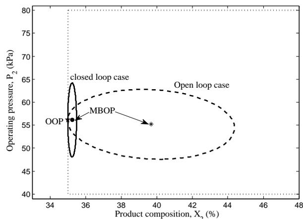
Fig. 3. Product composition vs operating pressure. a) Open loop case:  $F_3$  and  $F_{200}$  are constant. b) Closed loop case:  $F_3$  and  $F_{200}$  are used for control of  $X_2$
