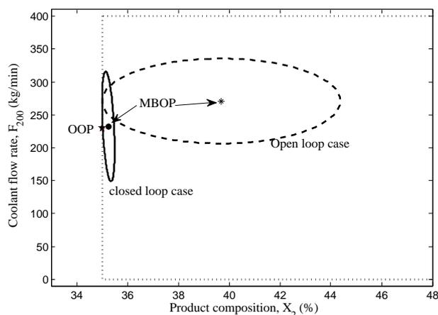
Fig. 6. Product composition vs coolant flow rate
