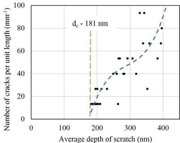
Fig. 10 Number of cracks per unit length vs. average depth of scratch along the scratch path (both start and end of the scratch).
