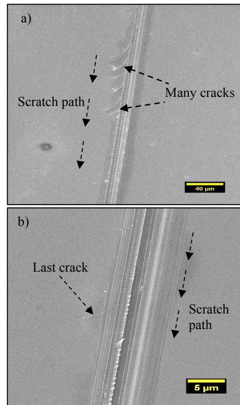
Fig. 8 a) SEM image shows many cracks in the transition region at the end of the scratch (T2); b) SEM image shows last crack in the transition region at the end of the scratch (T2).
