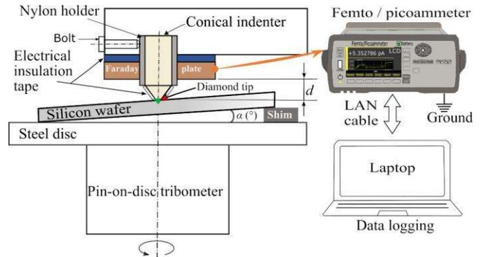
Fig. 3 Schematic of cross-sectional view of the experimental setup.
