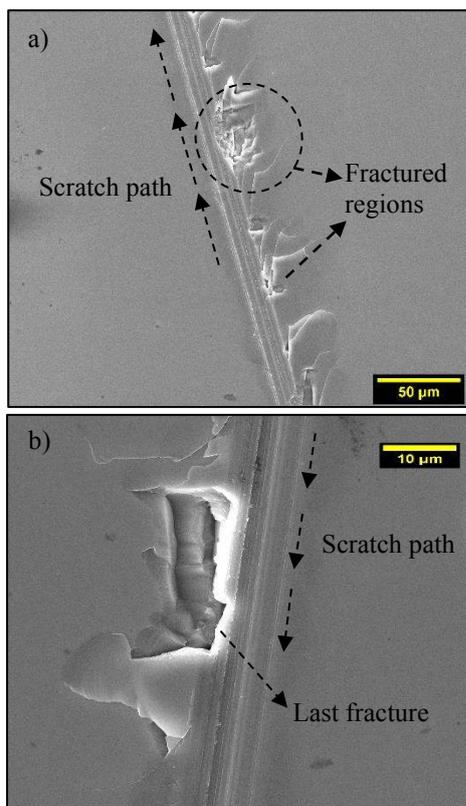
Fig. 7 a) SEM image shows fractured regions in the brittle region of the scratch (B); b) SEM image shows last fracture in the brittle region of the scratch (B).
