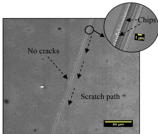
Fig. 9 SEM image of ductile region at the end of the scratch (D2).
