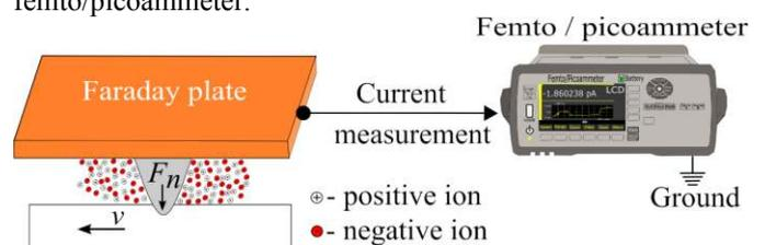
Fig. 1 CPE measurement during scratching.
