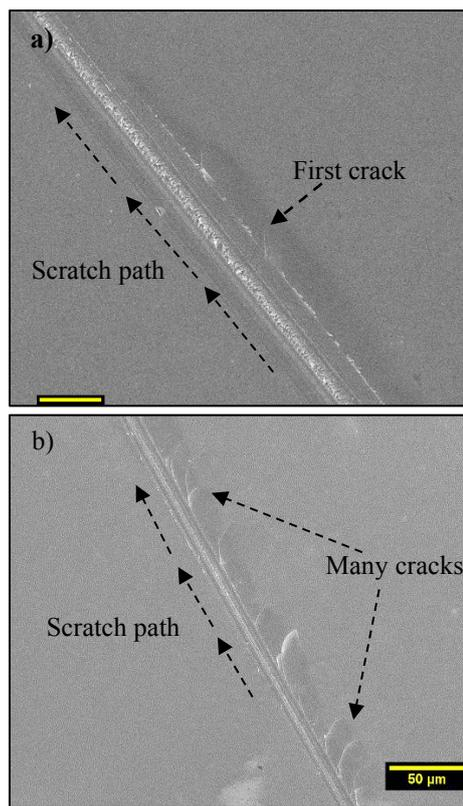
Fig. 6 a) SEM image shows first crack in the transition region at the start of the scratch (T1); b) SEM image shows many cracks in the transition region at the start of the scratch (T1).
