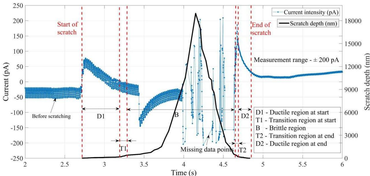
Fig. 4 Emission current intensity signal measured during the scratching process along with scratch depth (nm).
