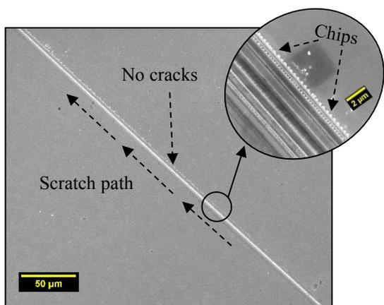
Fig. 5 SEM image of ductile region at the start of the scratch (D1).
