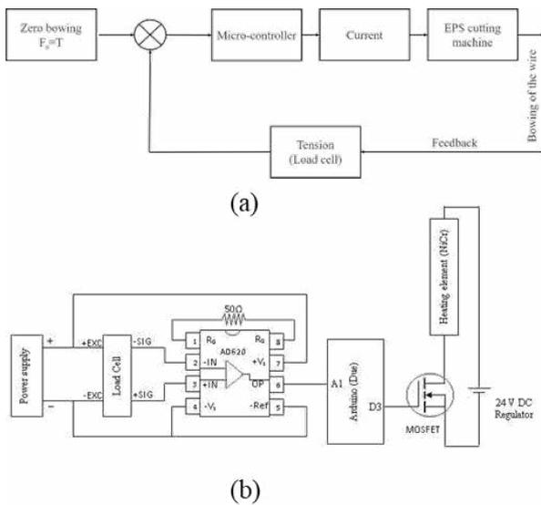
Figure 6 (a) Control block diagram of the wire-tension based feedback control developed (b)
