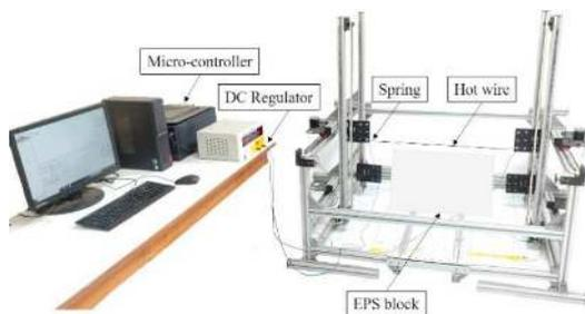
Figure 1. In-house built CNC hot wire cutting system.
