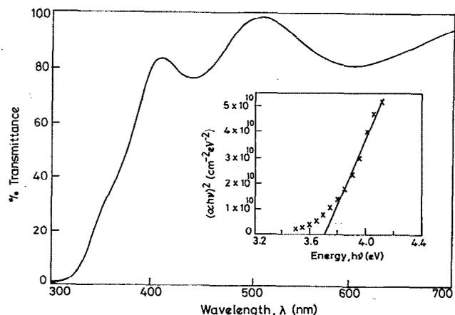
FIG. 2. Variation of transmittance as a function of wavelength for a typical indium oxide film. The inset shows a plot of  $(\alpha h\nu)^2$  against energy. The continuous line shows the least squares fit.
