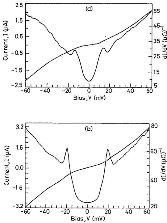
FIG. 3. (a) The  $I$ - $V$  characteristics together with the conductance data for a typical BSCCO junction and (b) the corresponding plot for the NBCO junction.
