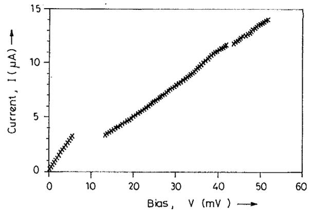
FIG. 4. The  $I$ - $V$  characteristics of a typical BSCCO junction with a 30-Å-thick barrier layer.
