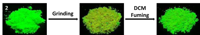
Fig. 6 Color changes of compound 2 upon grinding and fuming process under UV light irradiation at 365 nm.
