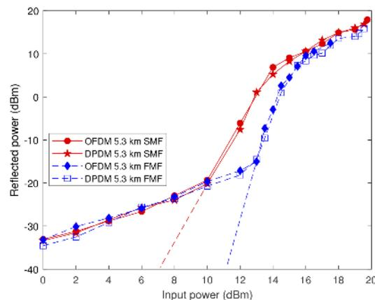
**Fig. 6.** Variation of reflected power with input power for same length of SMF and FMF (5.3 km).
