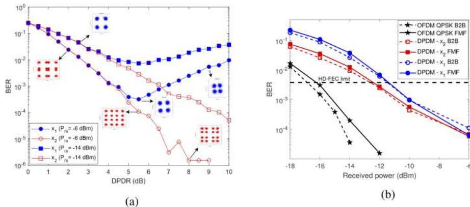
**Fig. 4.** (a) Variation of BER for  $\mathbf{x}_1$  and  $\mathbf{x}_2$  for different digital power division ratios and at different levels of received power in back-to-back condition (b) Variation of BER vs received power for the two DPDM channels and for QPSK-based DD-OFDM in back-to-back condition and in the presence of  $5.3$  km of FMF
