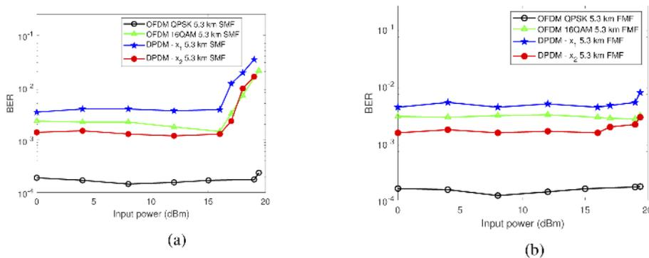
**Fig. 7.** Variation of BER with input power for same length (5.3 km) of (c) SMF and (d) FMF corresponding to of 5.3 km for QPSK-based DD-OFDM, 16QAM-based DD-OFDM and two-channel DPDM.
