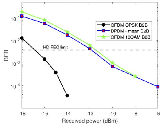
**Fig. 5.** Variation of mean BER of the two DPDM channels vs received power in back-to-back condition compared with that for QPSK-based OFDM and 16QAM-based OFDM
