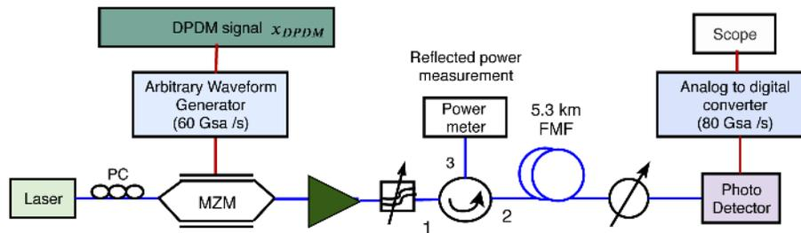
**Fig. 3.** Schematic of experimental set up for transmission of two-channel DPDM signal through 5.3 km of FMF
