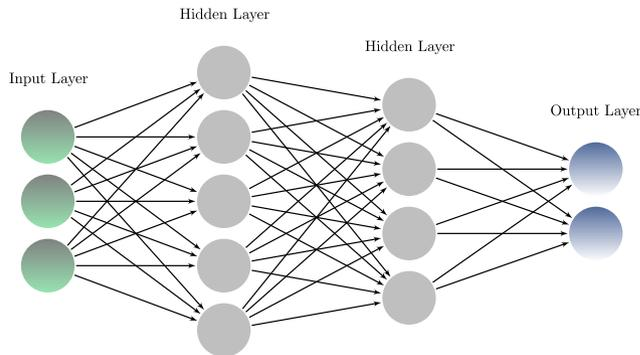
FIGURE 3 Schematic of a multilayer perceptron
