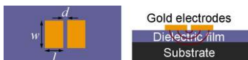
FIG. 3. Schematic views of the coplanar capacitor structure. Top view showing the dimensions (left side) and cross-sectional view showing the electric field lines through the dielectric film and the substrate (right side).
