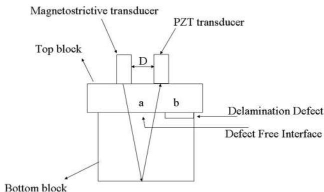
FIG. 6. Schematic diagram showing the ultrasonic pitch-catch technique.
