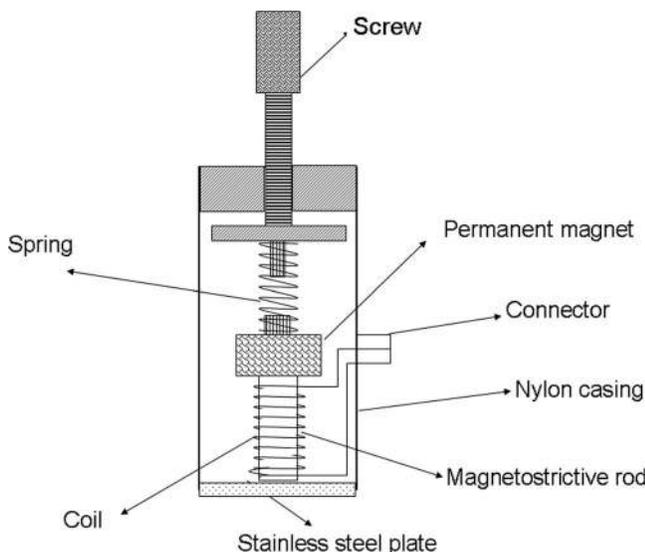
FIG. 2. Cross sectional view of the magnetostrictive transducer.
