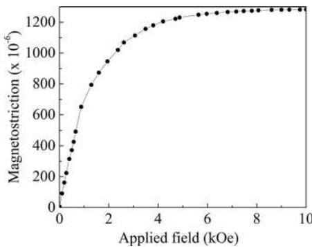
FIG. 1. Magnetostriction graph of Tb<sub>0.3</sub>Dy<sub>0.7</sub>Fe<sub>2</sub>.
