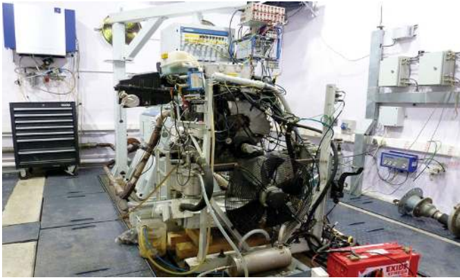
Figure 8. 250 kW transient dynamometer facility.
