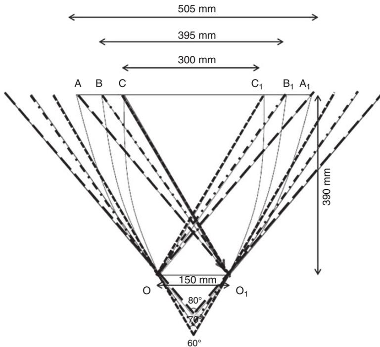
**Figure 4** Anidolic concentrators with uniform height but varying entry aperture size
