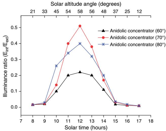
Figure 6 Performance of anidolic concentrators (uniform profile) under an overcast sky
