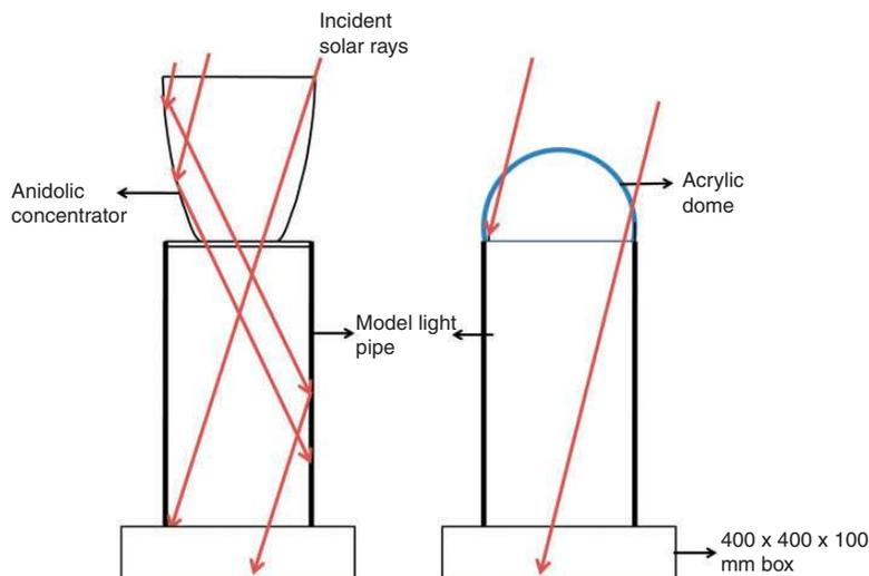
**Figure 5** Illustration of a light pipe with an anidolic concentrator and an acrylic dome
