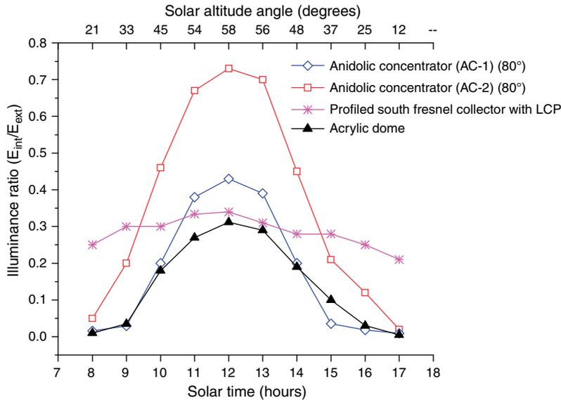
**Figure 9** Performance comparison of anidolic concentrators (acceptance angle 80°) with other collectors
