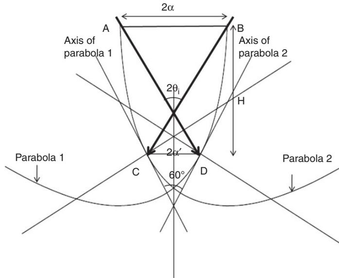
Figure 2 Construction of parabolae for an anidolic concentrator
