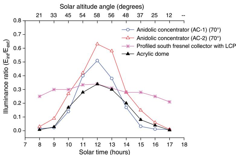
**Figure 8** Performance comparison of anidolic concentrators (acceptance angle  $70^\circ$ ) with other collectors
