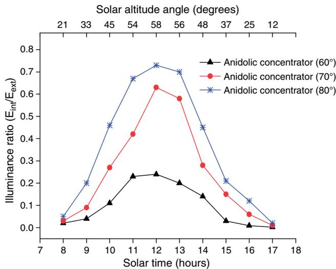
Figure 7 Performance of anidolic concentrators (uniform height) under an overcast sky
