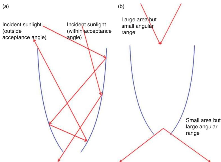
**Figure 1** An anidolic concentrator. (a) Concentrates light within its half acceptance angle. (b) Input aperture has larger area but smaller angular range.<sup>7</sup>
