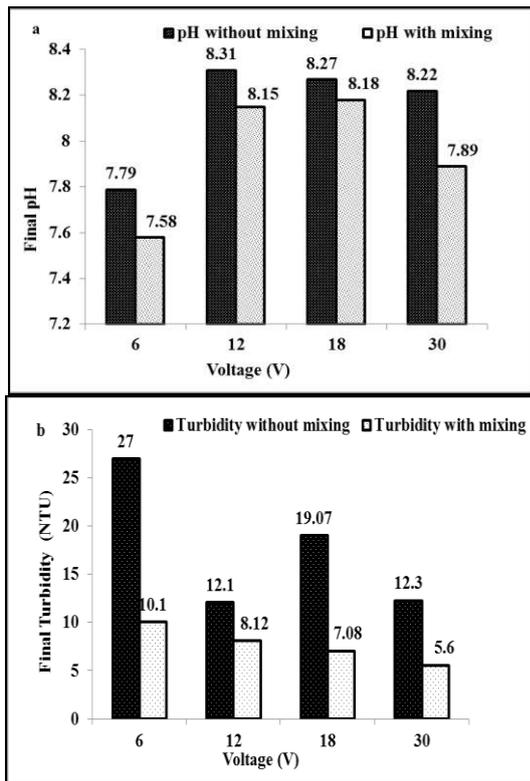
**Figure 6.** Effect of secondary mixing on final water pH (a) and turbidity (b) at different voltages for initial pH of 7.3 and initial turbidity of 175 NTU using Fe electrode
