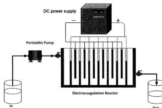
**Figure 1.** Schematic of the laboratory scale EC setup
