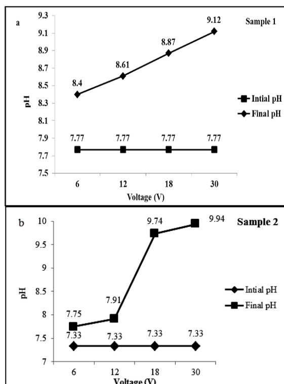
Figure 5. Effect of applied voltage on final water pH for sample 1 (initial turbidity of 391 NTU) (a) and sample 2 (initial turbidity of 175 NTU) turbidity removal (b) for Fe electrode
