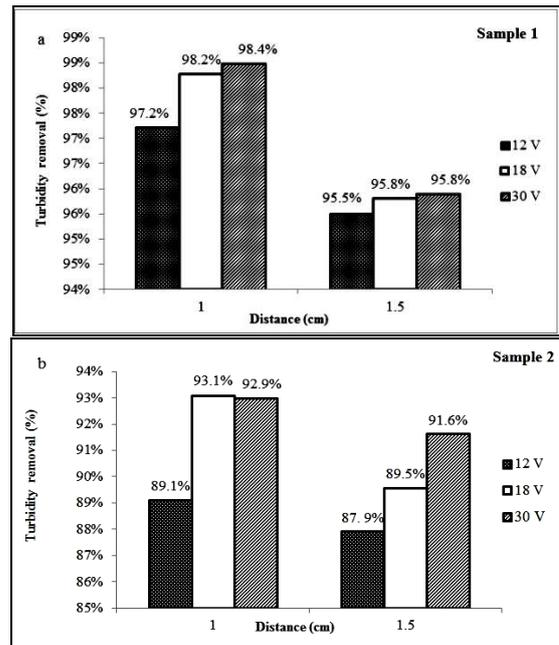
**Figure 3.** Effect of inter-electrode distance on turbidity removal for sample 1 (a) and sample 2 (b) for Fe electrode and different applied voltages: samples 1 and 2 represent turbidities of 391 and 175 NTU, respectively
