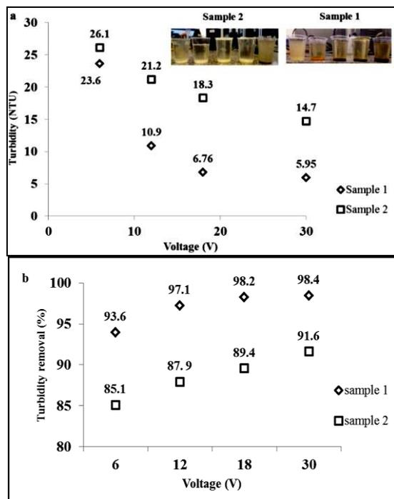
**Figure 2.** Effect of applied voltage on output turbidity (a) and turbidity removal (b) for Fe electrode and inter electrode distance of 1 cm: samples 1 and 2 represent turbidities of 391 and 175 NTU, respectively
