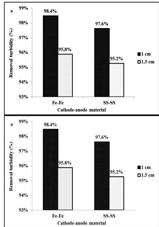
**Figure 4.** Turbidity removal for Fe-Fe and SS-SS electrodes (different anode electrode material) (a) and Fe-Fe and SS-Fe electrodes (constant anode material) (b) for sample 2 at different inter-electrode distances
